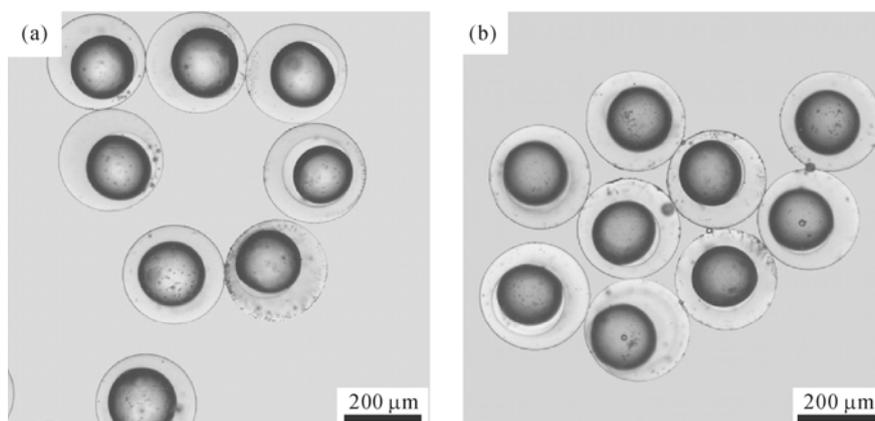
**Fig.2.** Optical micrographs of monodisperse microcapsules with pure oil core (a) and with Sudan III-loaded oil core (b) in water at 20 °C (Wang 2009).
