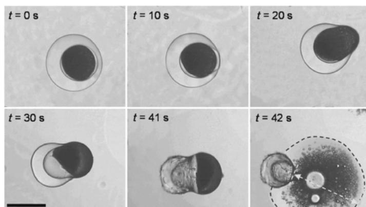
**Fig.8.** Microscope snapshots of thermo-triggered squirting of nanoparticles from microcapsules by increasing environmental temperature from 20 to 50 °C. The blue dashed line indicates the propagating front of the squirted liquid containing nanoparticles, and the yellow arrow shows the propagating distance of the squirted liquid containing nanoparticles (Liu 2010).
