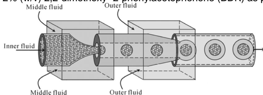
**Fig.5.** Schematic illustration of the microfluidic device (Liu 2010).
