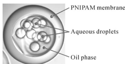
**Fig.10.** Optical micrograph of a typical Trojan-horse-like microcapsule consisting of a membrane of thermo-responsive PNIPAM hydrogel which encapsulates an oil drop containing several water droplets. The scale bar is 200  $\mu\text{m}$
