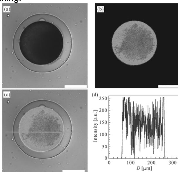
**Fig.7.** CLSM images of the prepared microcapsule at room temperature, in which (a) shows transmission channel image, (b) shows green channel image and (c) shows the overlay of green channel and transmission channel images. Scale bars are 100  $\mu\text{m}$ . (d) Fluorescence intensity profile corresponding to (c) (Liu 2010).
