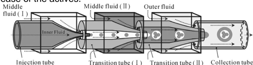
**Fig.9.** Schematic diagram of the capillary microfluidic device for generating triple emulsions (Chu 2007).
