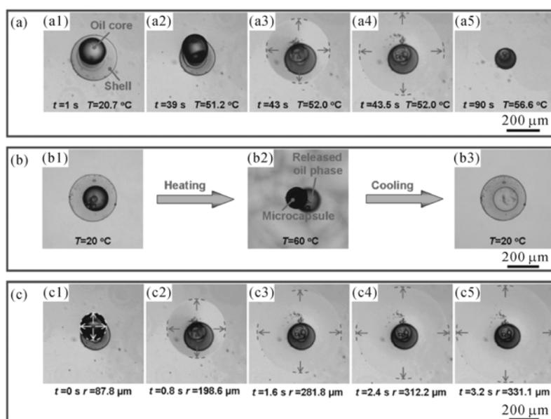
**Fig.3.** Optical microscope snapshots of the thermo-induced self-bursting behavior (a) and complete release performance (b) of the as-prepared microcapsules. (c) Thermo-induced burst-release process of inner oil core from the microcapsule (shown in (a)) during the first 3.2 s of release, in which time-dependent increase of the radius ( $r$ ) of the circle edge of released oil phase is used to evaluate the release rate (Wang 2009).
