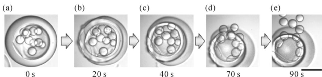
**Fig.11.** Optical micrograph time-series showing the forced expulsion of the oil and water droplets contained within the PNIPAM microcapsule when the temperature is rapidly increased from 25 °C to 50 °C. The scale bar is 200  $\mu\text{m}$  (Chu 2007).
