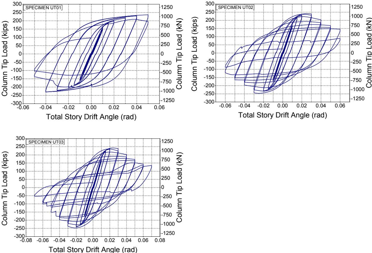
Fig. 3 Column tip load versus total story drift angle for all specimens
