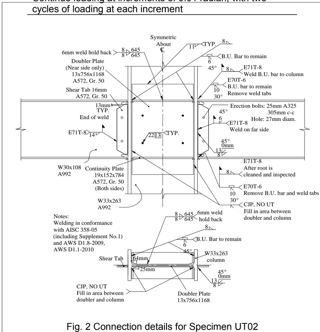
Fig. 2 Connection details for Specimen UT02
