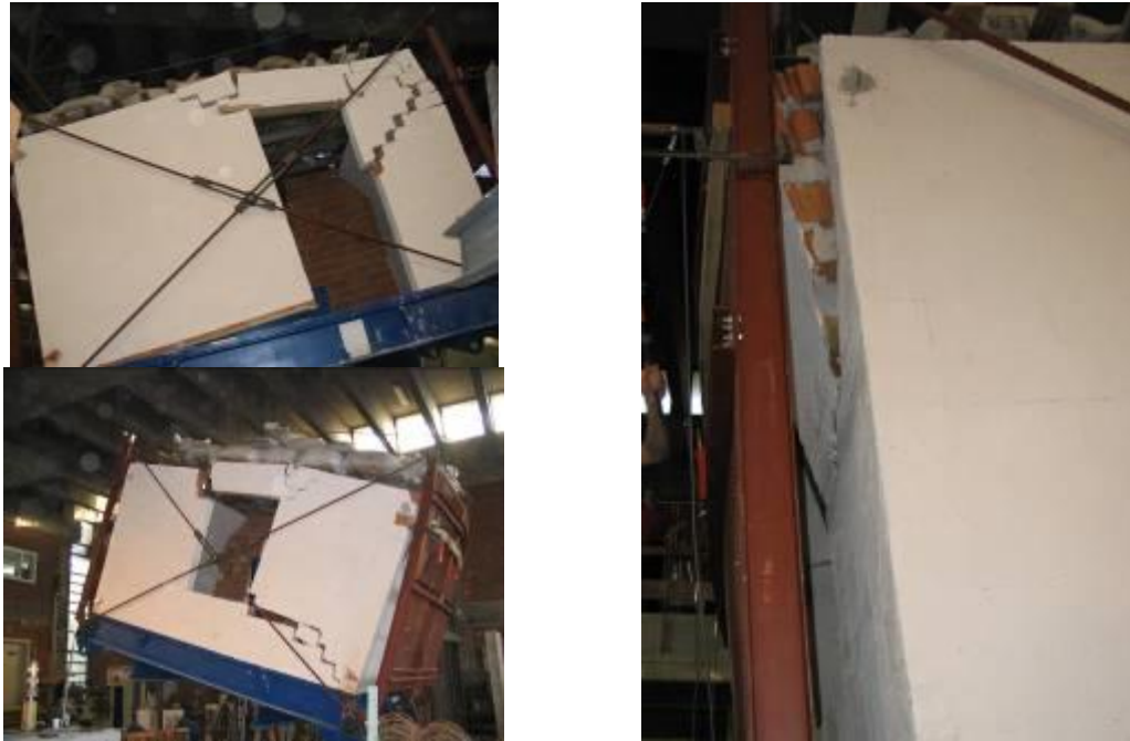
Fig. 14 Failure of original masonry house at an angle of 18^\circ
