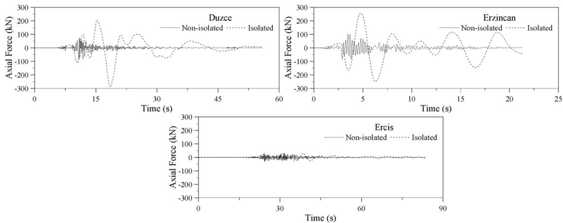
Fig. 6. Maximum axial force of cable  $A_1$ .
