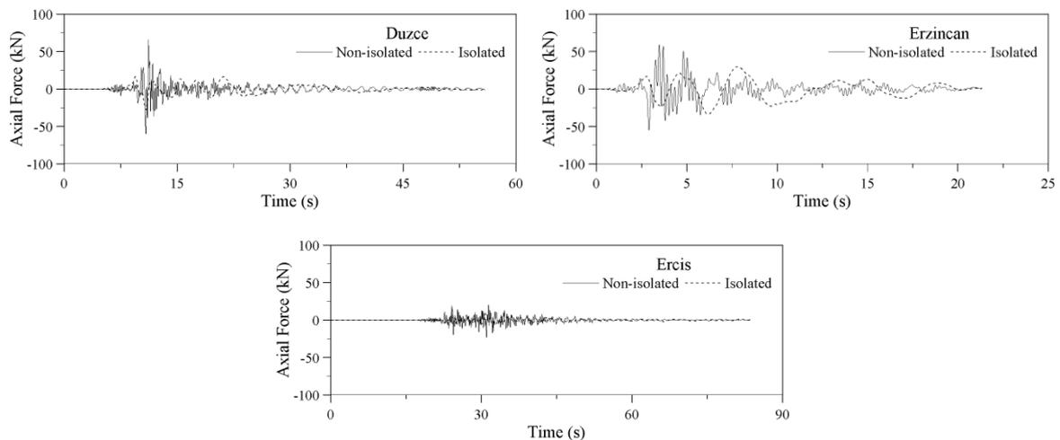
Fig. 9. Maximum axial force of cable A<sub>4</sub>.
