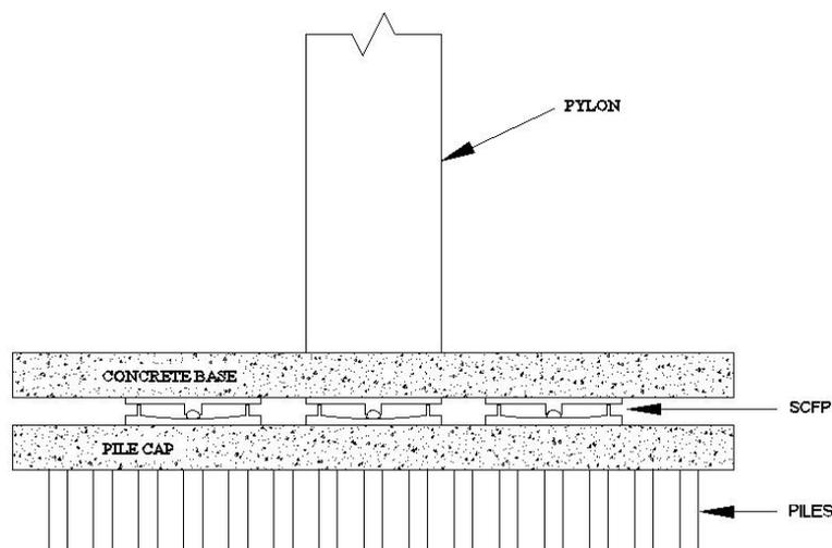
Fig 3 Location of SCFP bearings at the pylon-foundation connection
