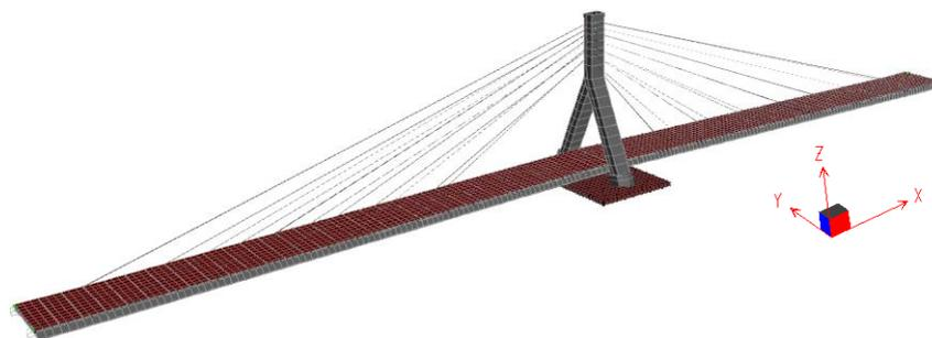
Fig. 4 Finite Element Model of Manavgat Cable-Stayed Bridge
