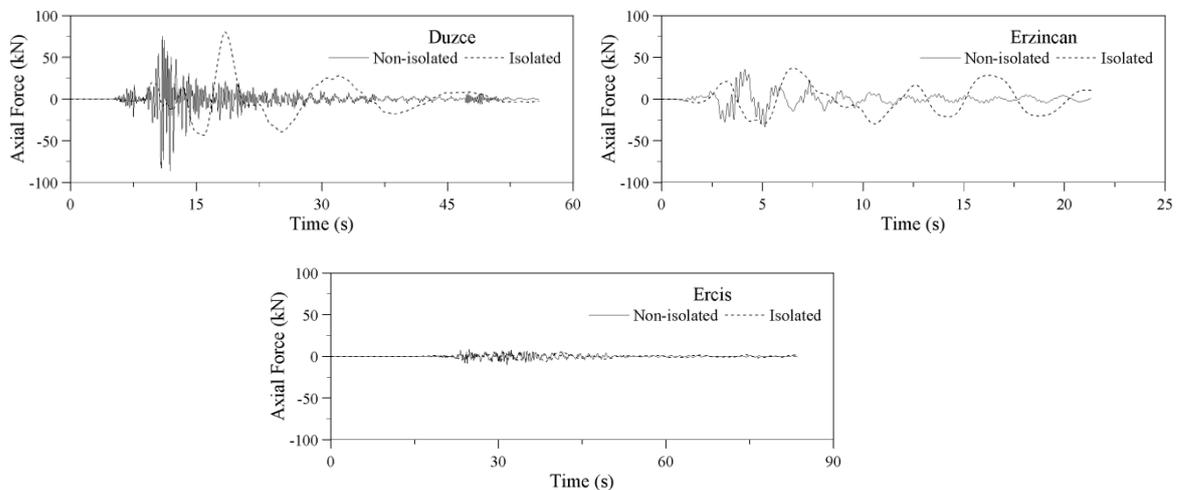
Fig. 11. Maximum axial force of cable  $A_6$ .
