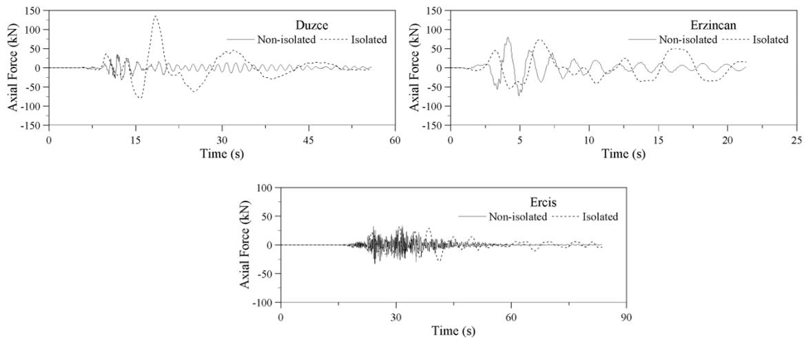
Fig. 12. Maximum axial force of cable A<sub>7</sub>.
