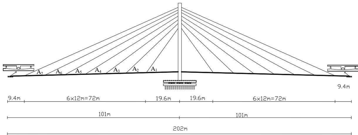
Fig 2 The schematic form of Manavgat Cable-Stayed Bridge
