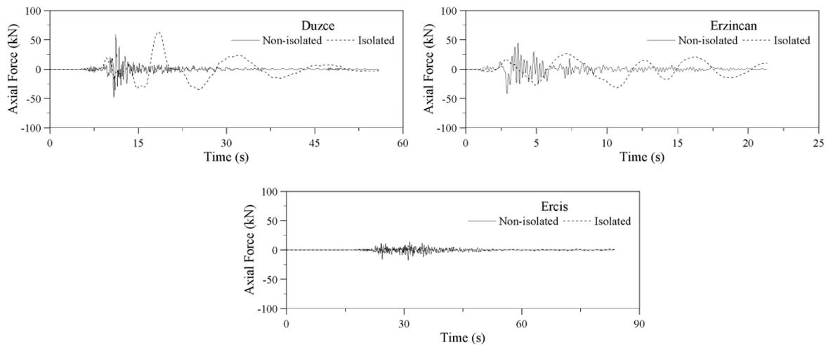
Fig. 10. Maximum axial force of cable  $A_5$ .
