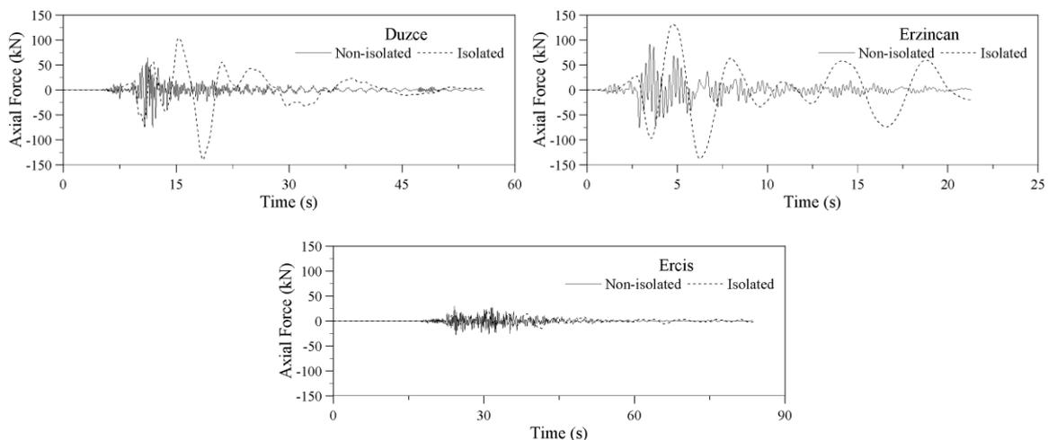
Fig. 7. Maximum axial force of cable  $A_2$ .
