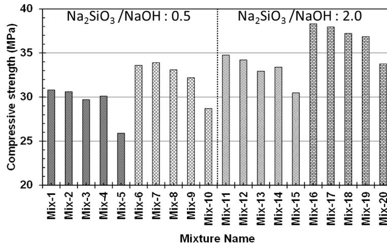
**Fig. 4.** Compressive strength by the ratio of  $\text{Na}_2\text{SiO}_3$  to NaOH
