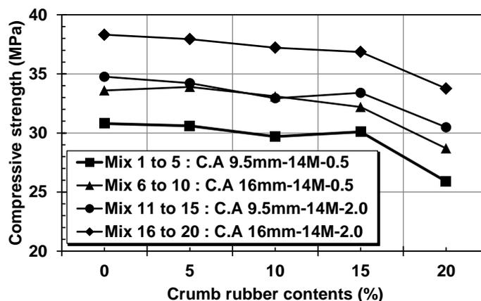
**Fig. 5.** Compressive strength by amount of crumb rubber
