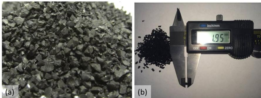
**Fig. 1.** (a) Crumb rubber and (b) Particle size of crumb rubber
