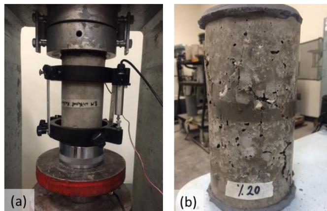
**Fig. 3.** (a) Compressive strength test set up and (b) Failure of cylinders (20%: rubber)
