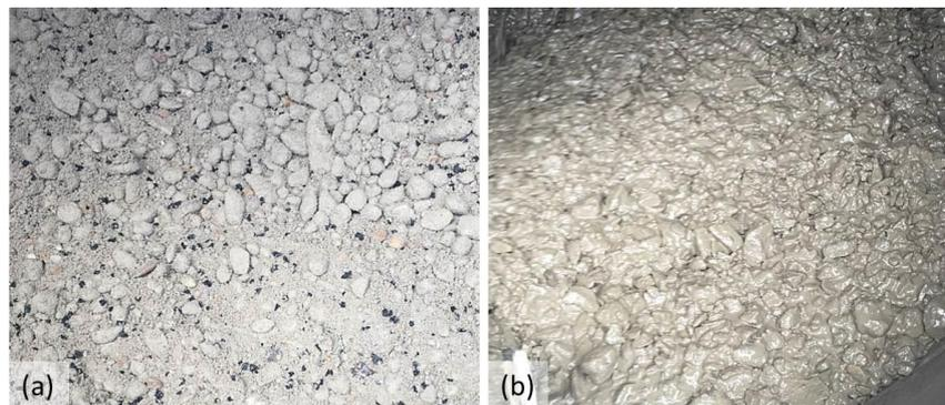
**Fig. 2.** (a) Mix without alkaline solutions and (b) Mix with alkaline solutions (20% rubber)
