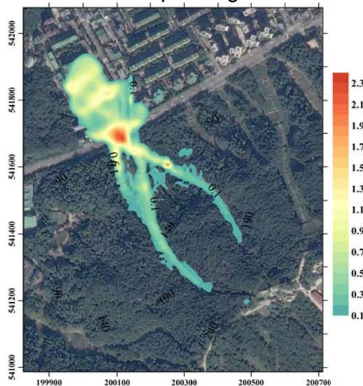
Fig.2 Propagation and maximum flow depth
