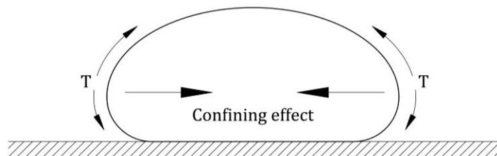
Fig. 16 Geotextile tube's confining effect
