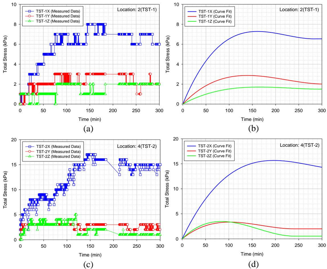
Fig. 15 (a) Total stress readings at Location ②; (b) curve fit for the stress readings at Location ②; (c) total stress readings at Location ④; (d) curve fit for the stress readings at Location ④;
