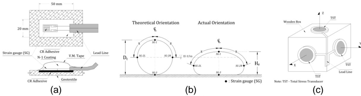
Fig. 4. (a) Strain gauge installation details; (b) strain gauge positioning on the geotextile tube, and; (c) total stress transducer contraction.
