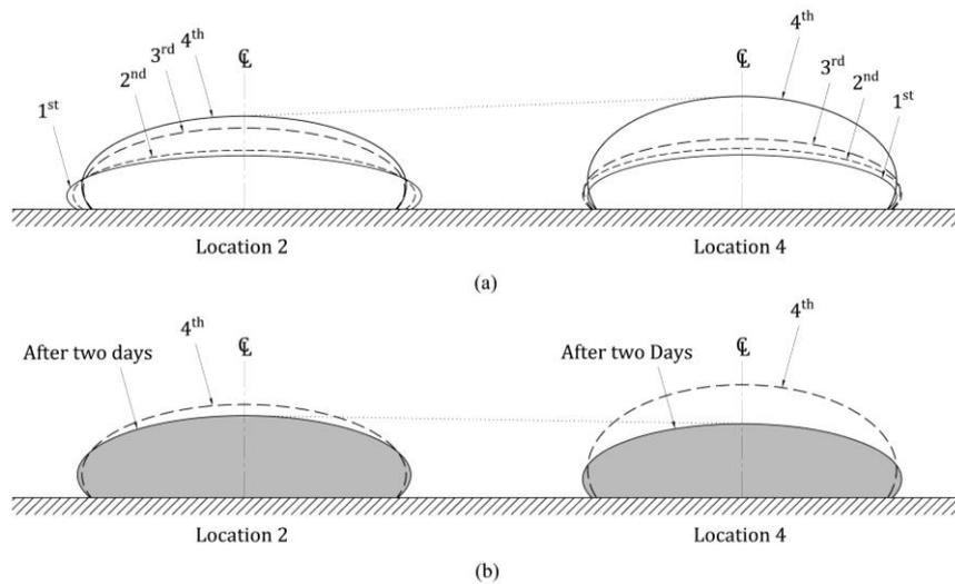
Fig. 7 Geotextile tube shape variation: (a) during filling stages; (b) stabilized stage – two days after the last filling stage
