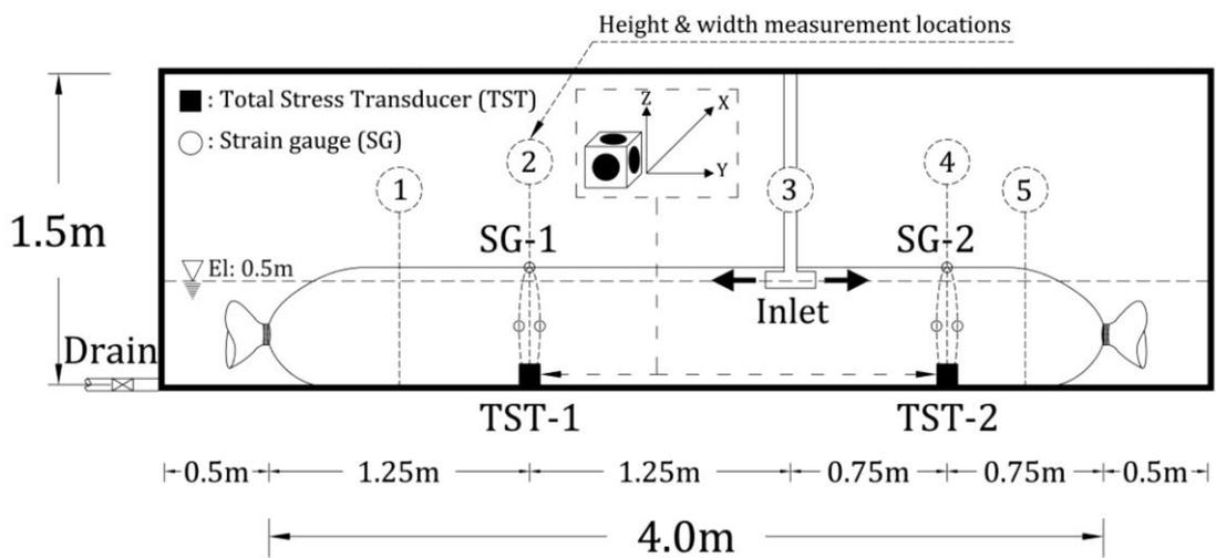
Fig. 5. Instrumentation placement
