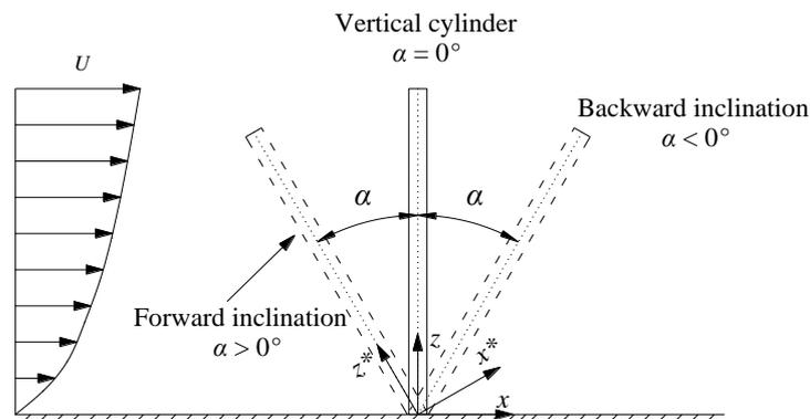
Fig. 4 Illustration of tested three different types of cylinders: the forward inclined cylinder, the vertical cylinder, and the backward inclined cylinder.  $\alpha$  is the angle of inclination: a positive value represents the forward inclination while a negative one denotes the backward inclination.
