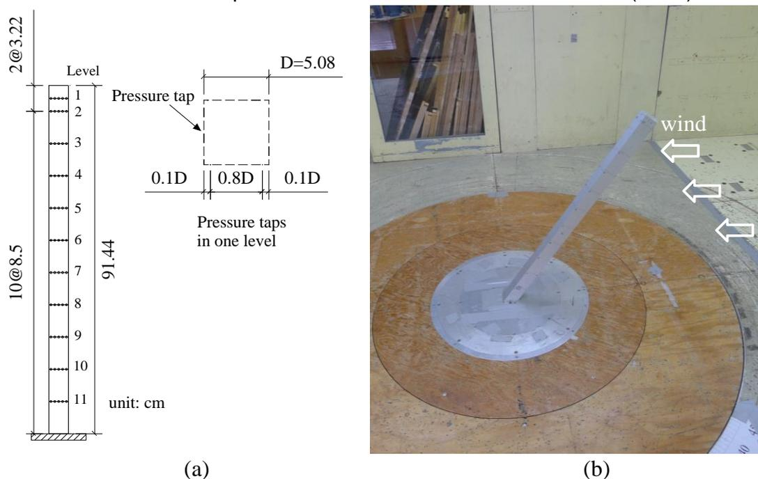
Fig. 5A model for wind tunnel pressure measurements: (a) the tested model dimensions and the distribution of pressure taps, (b) a square-section cylinder with a forward inclination angle in the wind tunnel.
