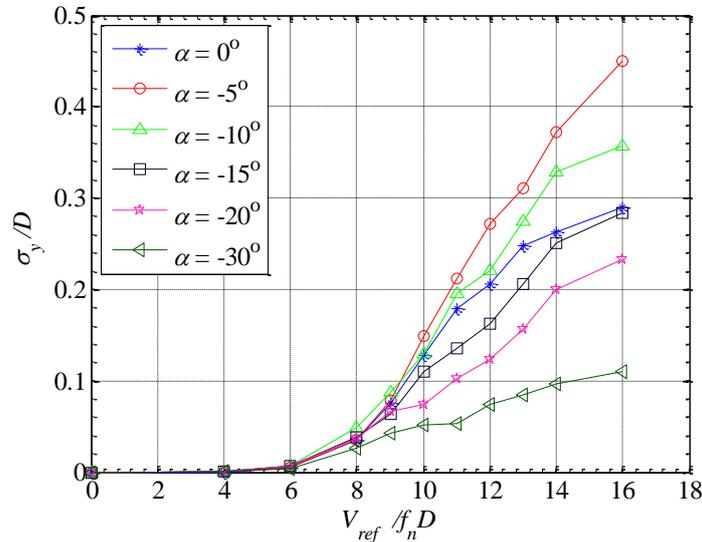
Fig. 7 Across-wind responses of backward inclined cylinders compared with the vertical cylinder.
