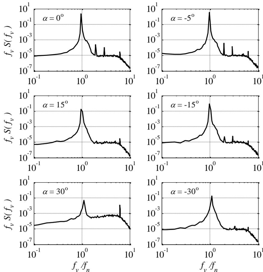
Fig. 8 Power spectra of across-wind responses of the cylinders at  $V_{red}=11$ .
