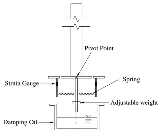
Fig. 3 Schematic of the aeroelastic model used in the wind tunnel tests.
