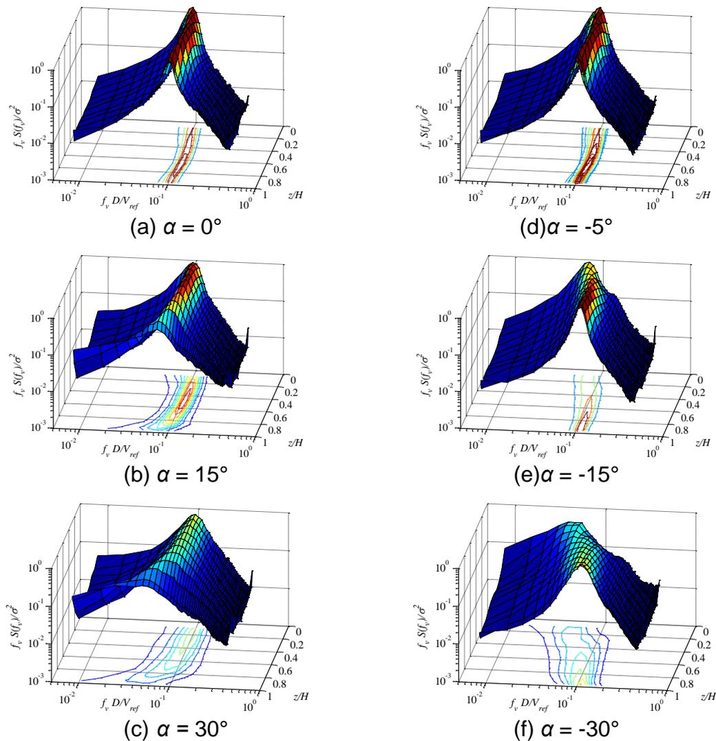
Fig. 9 Power spectra of pressures on the side face of the cylinders
