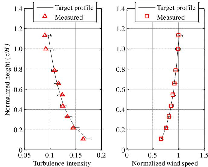
Fig. 2 Turbulent wind flow field adopted in the wind tunnel tests.
