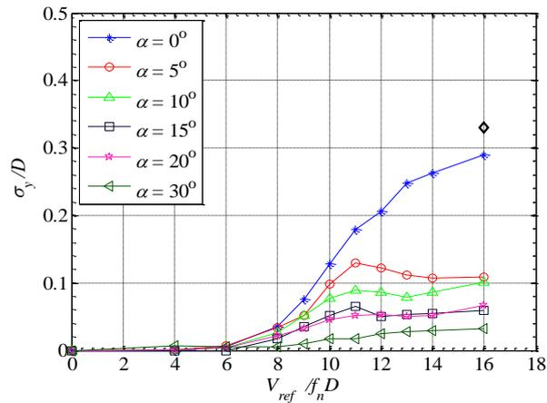
Fig. 6 Across-wind responses of forward inclined cylinders compared with the vertical cylinder.  $\diamond$ : transverse amplitude of a vertical cylinder with  $H/D= 18$ , damping ratio of 0.64%, and turbulence intensity of 9%(Kwok and Melbourne, 1980).
