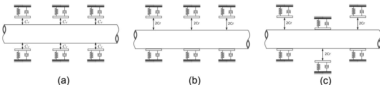
**Figure 8: Tube support offset types: (a) zero offset, (b) one-side offset, (c) alternating offset**
