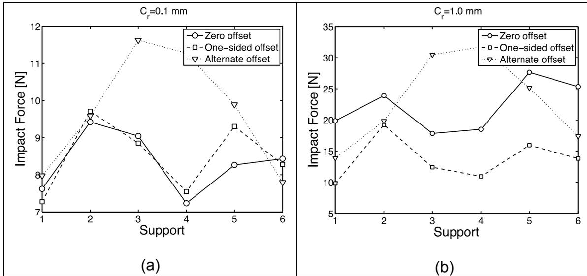
**Figure 10: The effect of the support offset on the rms impact force: (a) 0.1 mm clearance, (b) 1.0 mm clearance**
