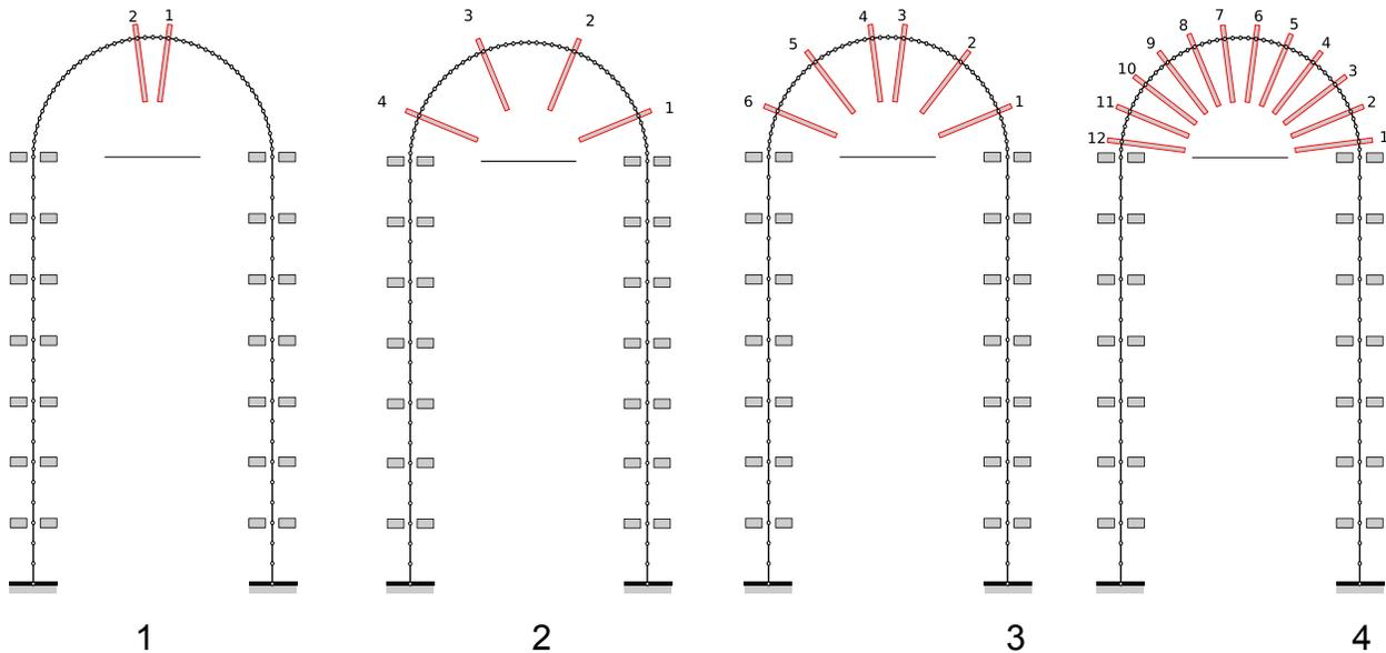
**Figure 4: Tube support configurations with different number of flat bar supports**
