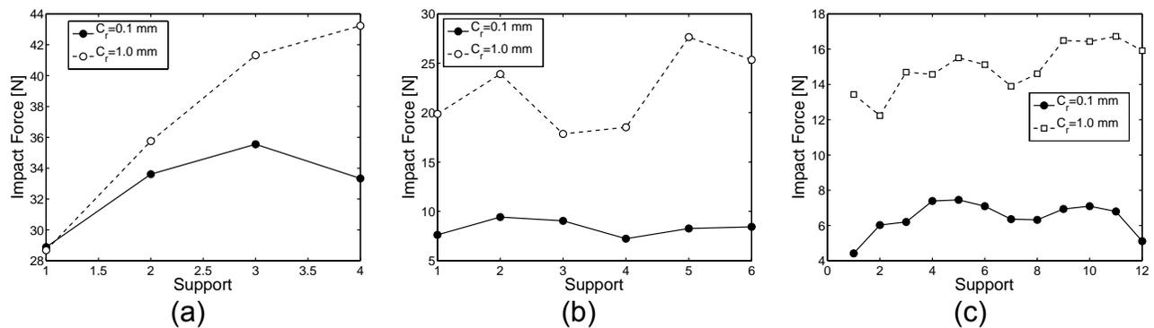
**Figure 6: rms impact force at the supports located in the U-bend: (a) Configuration 2, (b) Configuration 3, (c) Configuration 4**
