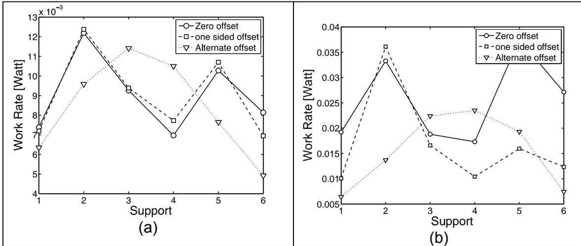
**Figure 11: The effect of the support offset on the normal work rate: (a) 0.1 mm clearance, (b) 1.0 mm clearance**
