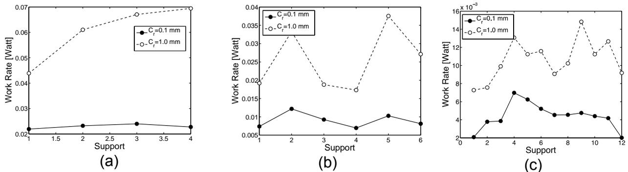
**Figure 7: Normal work rate at the supports located in the U-bend: (a) Configuration 2, (b) Configuration 3, (c) Configuration 4**
