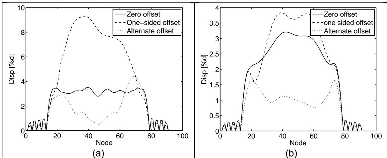
**Figure 9: The effect of the support offset on the response along the tube nodes: (a) transverse, (b) streamwise**
