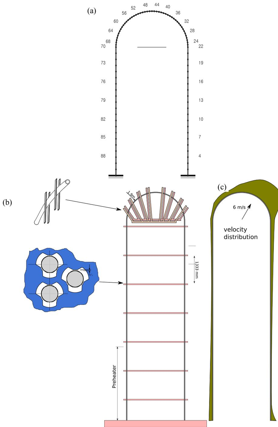
**Figure 3: U-bend tube configuration showing: (a) FE nodes along the U-bend, (b) Tube broached hole and flat bar supports, as well as (c) The flow distribution in the U-bend region**
