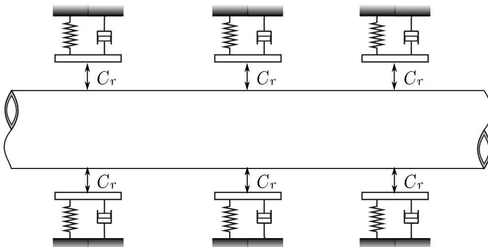
**Figure 1: Tube-support model**
