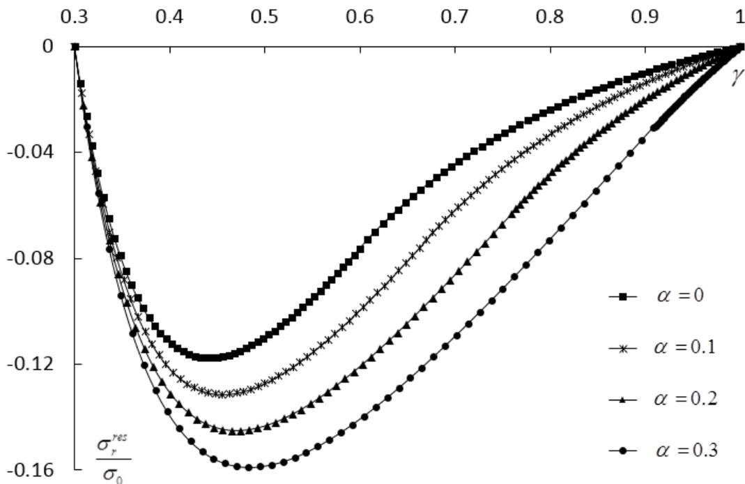
Figure 17. Variation of the residual radial stress with  $\gamma$  at  $\nu=0.3$ ,  $a=0.3$ ,  $\Omega_f=2.05$  and several  $\alpha$ - values.
