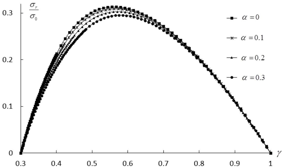
Figure 9. Variation of the radial stress with  $\gamma$  at  $\nu=0.3$ ,  $a=0.3$ ,  $\Omega=1.62$  and several  $\alpha$ - values.
