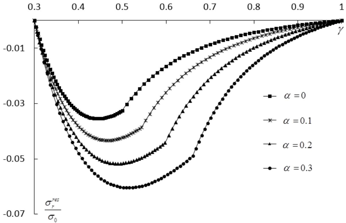
Figure 16. Variation of the residual radial stress with  $\gamma$  at  $\nu=0.3$ ,  $a=0.3$ ,  $\Omega_f=1.88$  and several  $\alpha$ - values.
