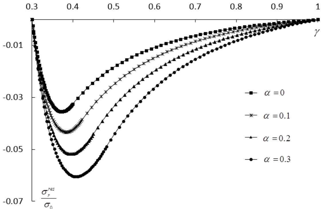
Figure 15. Variation of the residual radial stress with  $\gamma$  at  $\nu=0.3$ ,  $a=0.3$ ,  $\Omega_f=1.62$  and several  $\alpha$ - values.
