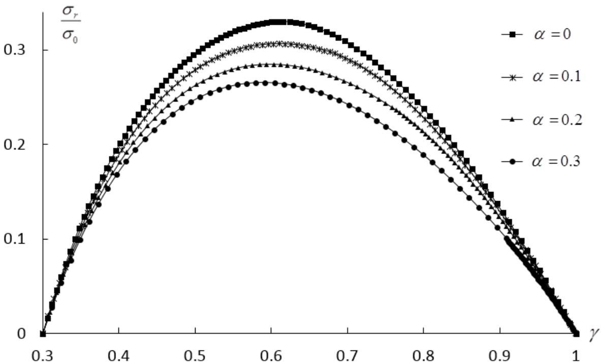
Figure 11. Variation of the radial stress with  $\gamma$  at  $\nu=0.3$ ,  $a=0.3$ ,  $\Omega=2.05$  and several  $\alpha$  - values.
