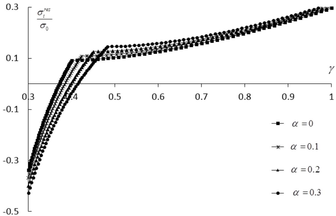
Figure 18. Variation of the residual circumferential stress with  $\gamma$  at  $\nu=0.3$ ,  $a=0.3$ ,  $\Omega_f=1.62$  and several  $\alpha$  – values.
