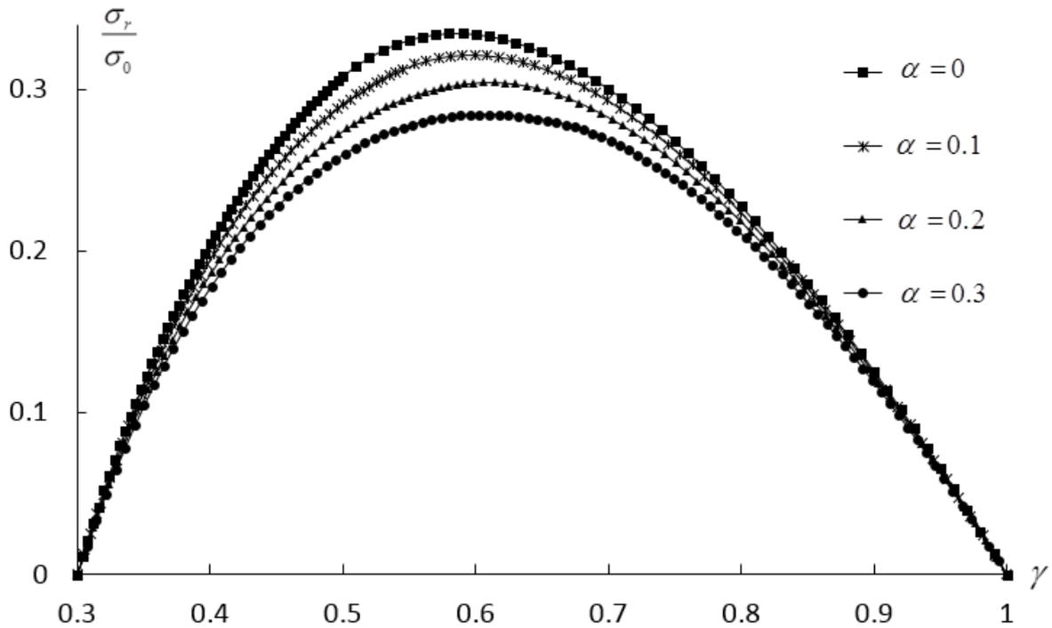
Figure 10. Variation of the radial stress with  $\gamma$  at  $\nu=0.3$ ,  $a=0.3$ ,  $\Omega=1.88$  and several  $\alpha$  - values.
