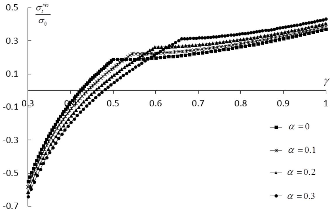
Figure 19. Variation of the residual circumferential stress with  $\gamma$  at  $\nu=0.3$ ,  $a=0.3$ ,  $\Omega_f=1.88$  and several  $\alpha$  – values.
