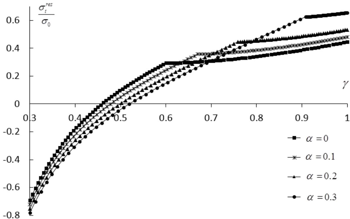
Figure 20. Variation of the residual circumferential stress with  $\gamma$  at  $\nu=0.3$ ,  $a=0.3$ ,  $\Omega_f = 2.05$  and several  $\alpha$  – values.
