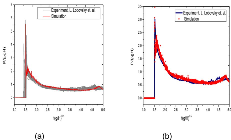
Fig. 8 The comparison of the non-dimensional pressure with the non-dimensional time at sensor 1 (a) between the simulation results with the 100 test of experiment data (b) between the simulation results with the average pressure from the experimental
