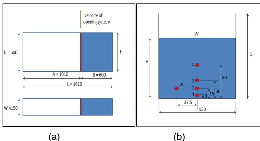
Fig. 6 The dam break simulation with an opening gate which corresponding to the experiment conducted by Lobovsky (2014)
