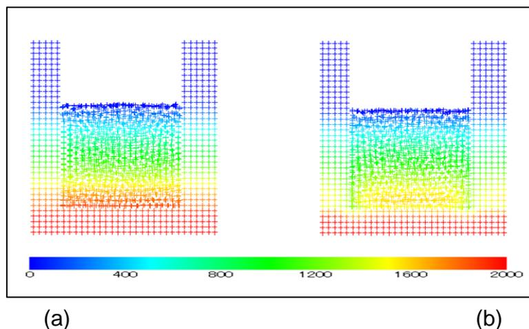
Fig. 2 The pressure distribution on the water particles and wall boundary by (a) using MVMRG with perfectly Neumann condition and (b) Pseudo Neumann boundary condition for compatible surface boundary
