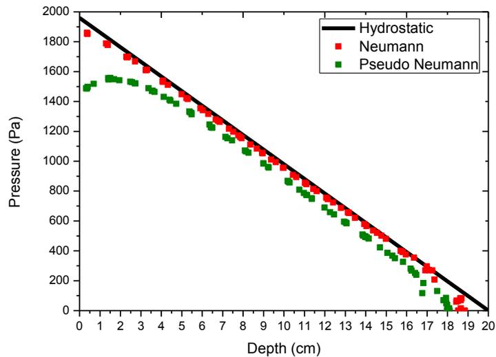
Fig. 3 The comparison of pressure distribution with the depth by using hydrostatic pressure, perfectly Neumann boundary treatment and Pseudo Neumann boundary condition for compatible surface boundary
