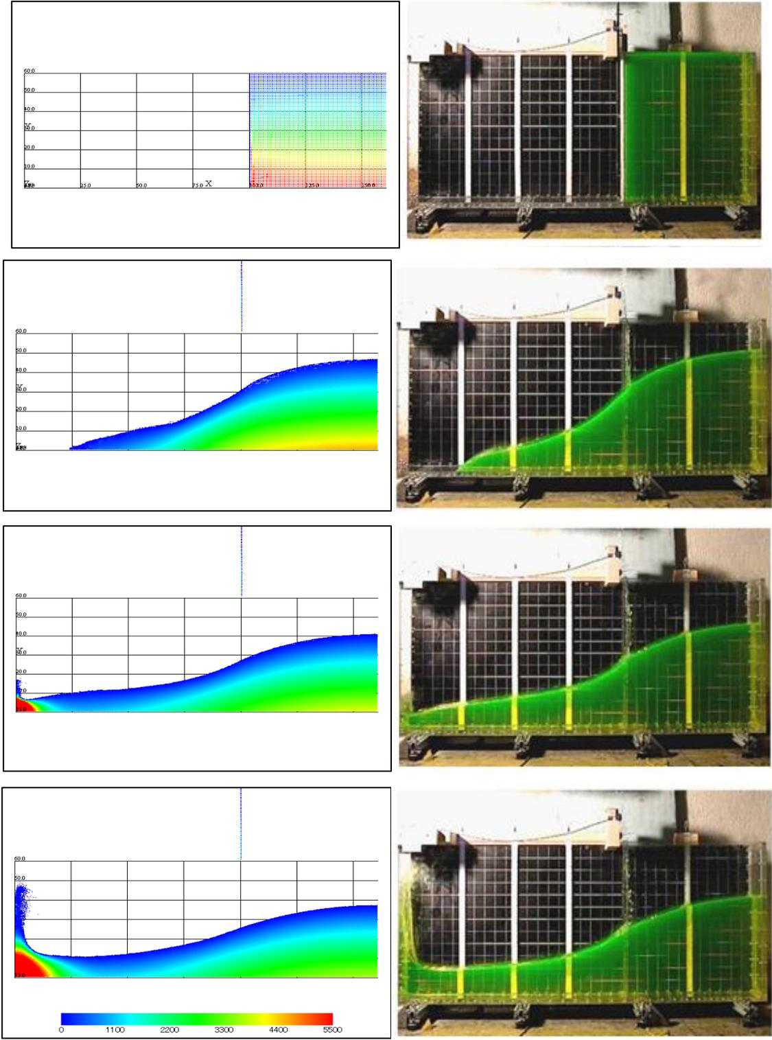
Fig. 7 The comparison of the free surface evolution between simulation and experimental at times 0.0, 316.7, 413.4, 463.3, and  $\pm 3.3$ ms
