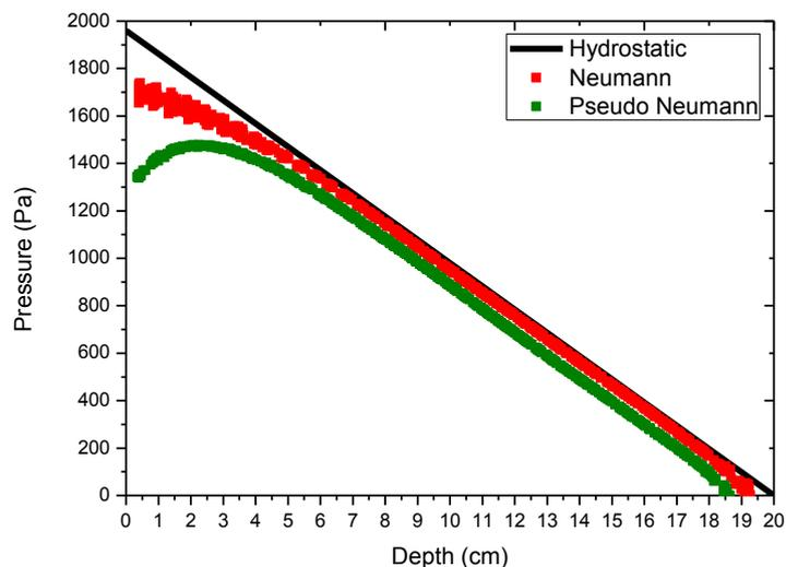
Fig. 5 The comparison of pressure distribution by using MVMRG with perfectly Neumann condition and Pseudo Neumann condition with the theoretical value hydrostatic pressure for compatible surface with complex geometrical objects
