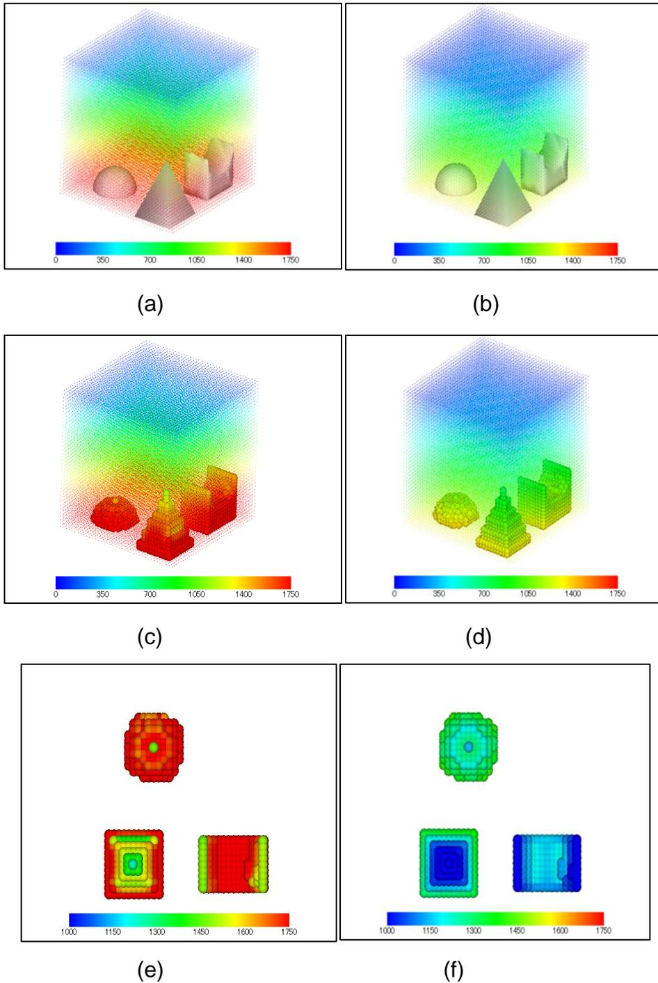
Fig. 4 The comparison of the pressure distribution using the modified boundary treatment which satisfied Neumann boundary condition with the treatment using Pseudo Neumann boundary condition: (a) the real shape of complex geometrical objects with pressure distribution of water using MVMRG with perfectly Neumann condition, (b) the
