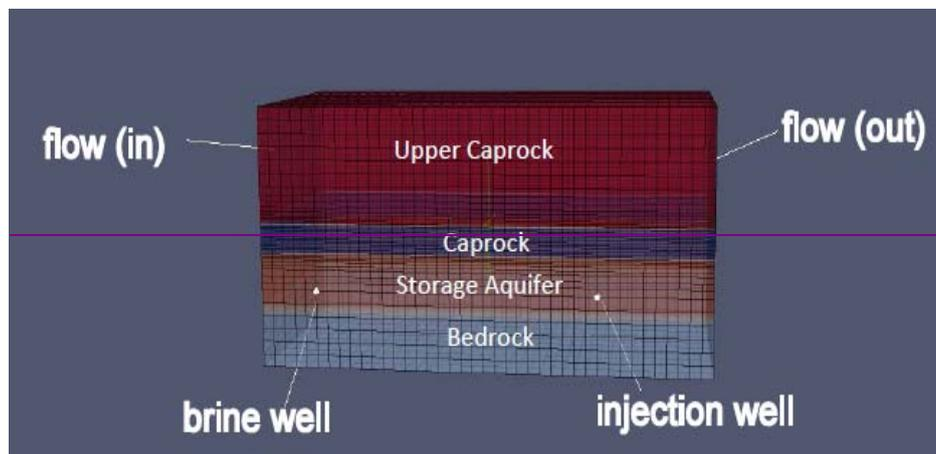
Fig. 4 Caprock leakage model and flow boundary condition
