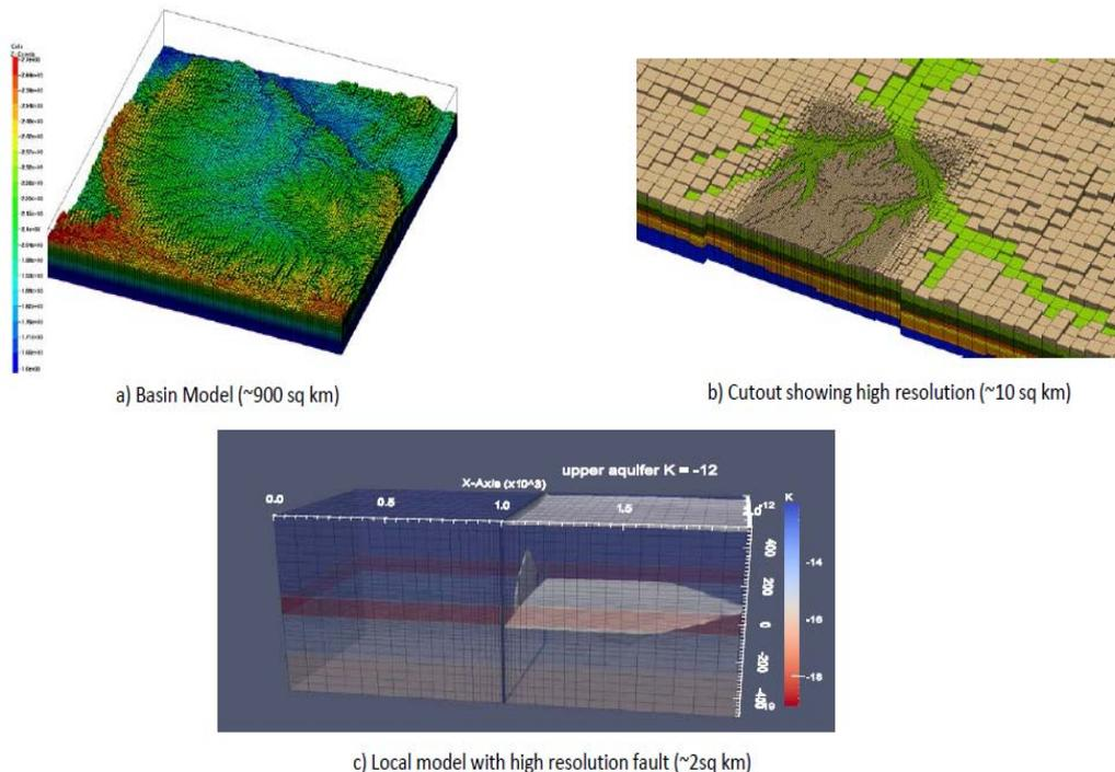
Fig. 2 Example of large scale reservoir model with an embedded high resolution model
