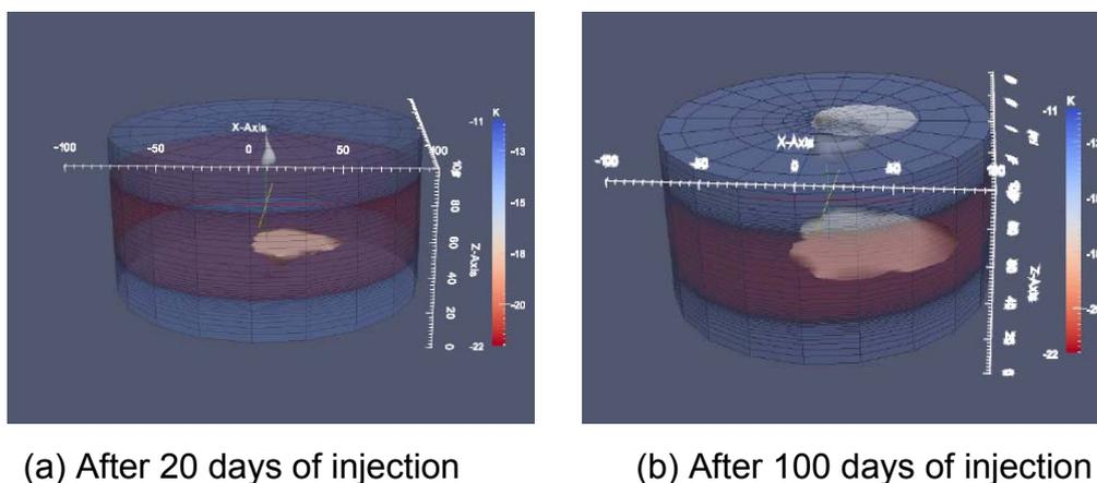
Fig. 9 CO<sub>2</sub> plume (Case 2\_Wellbore Leakage model)
