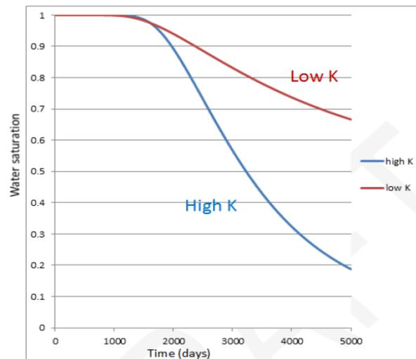
Fig. 12 Water saturation change for different upper aquifer permeability
