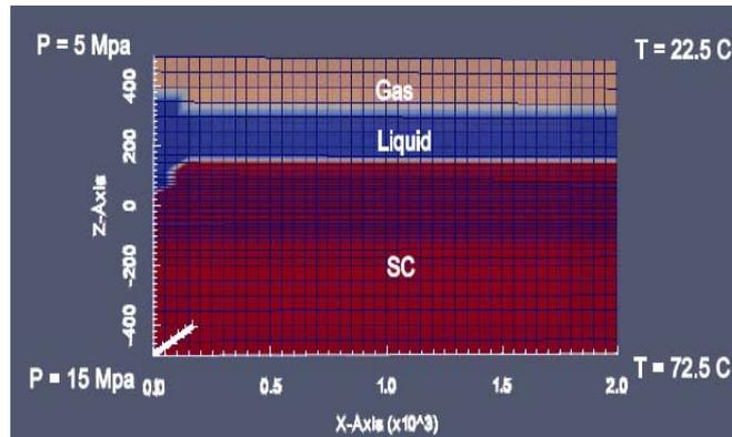
Fig. 7 CO<sub>2</sub> phase regions in subsurface with hydrostatic pressure and 0.05 °C/m temperature gradient
