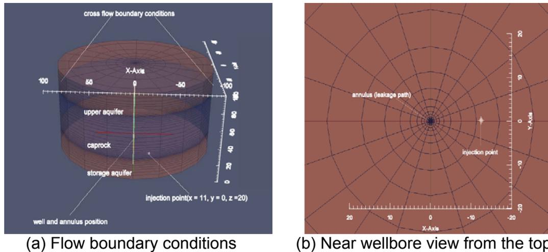
Fig. 3 Wellbore leakage model
