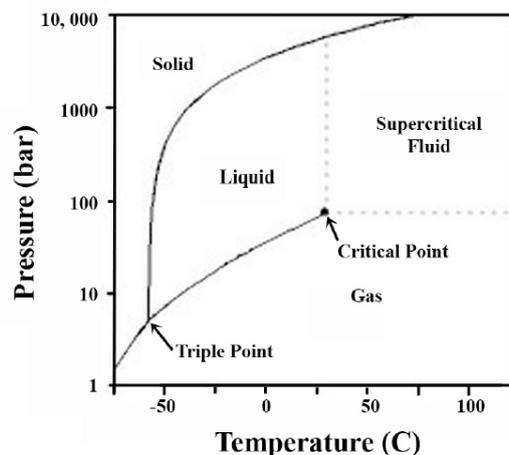
Fig. 6 CO<sub>2</sub> phase diagram (1 bar = 0.1 MPa)
