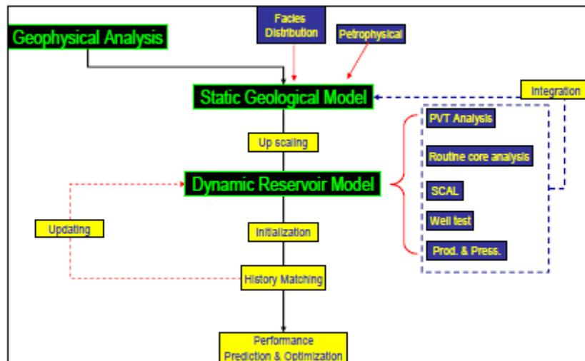
Fig. 4 Reservoir simulation workflow (LAPI ITB, 2010)
