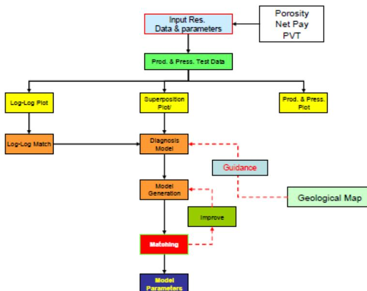
**Fig. 3** Pressure transient analysis workflow (LAPI ITB, 2010)
