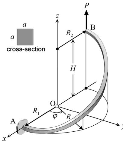
Fig. 1 The cantilevered conical helicoidal rod
