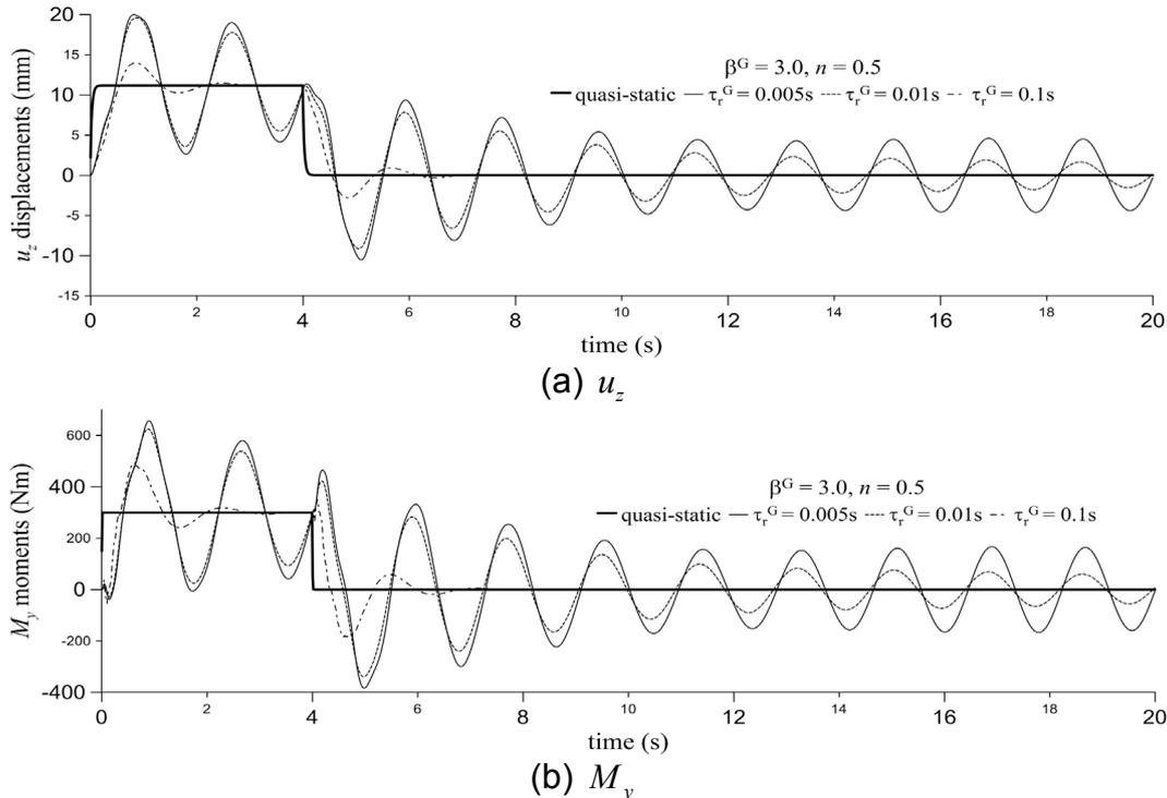
Fig. 2 Time histories of viscoelastic conical helicoidal rod subjected to the rectangular impulsive type load
