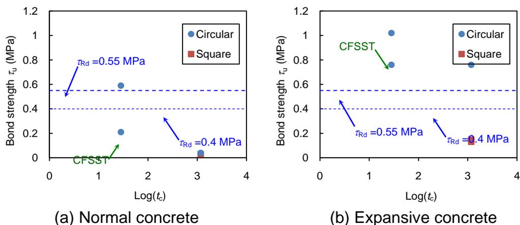
Fig. 7 Comparison between measured  $\tau_u$  and specified  $\tau_{Rd}$
