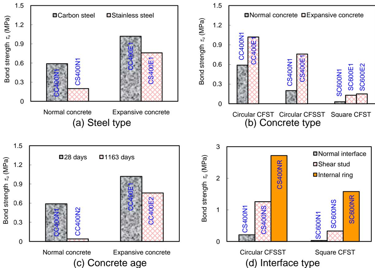
Fig. 6 Effects of different parameters on  $\tau_u$  between the steel tube and concrete.
