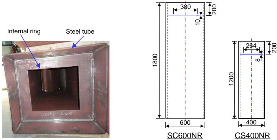
(a) Internal ring in specimen SC600NR      (b) Location of the internal ring
