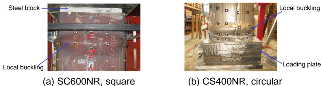
Fig. 4 Failure mode of specimens with an internal ring
