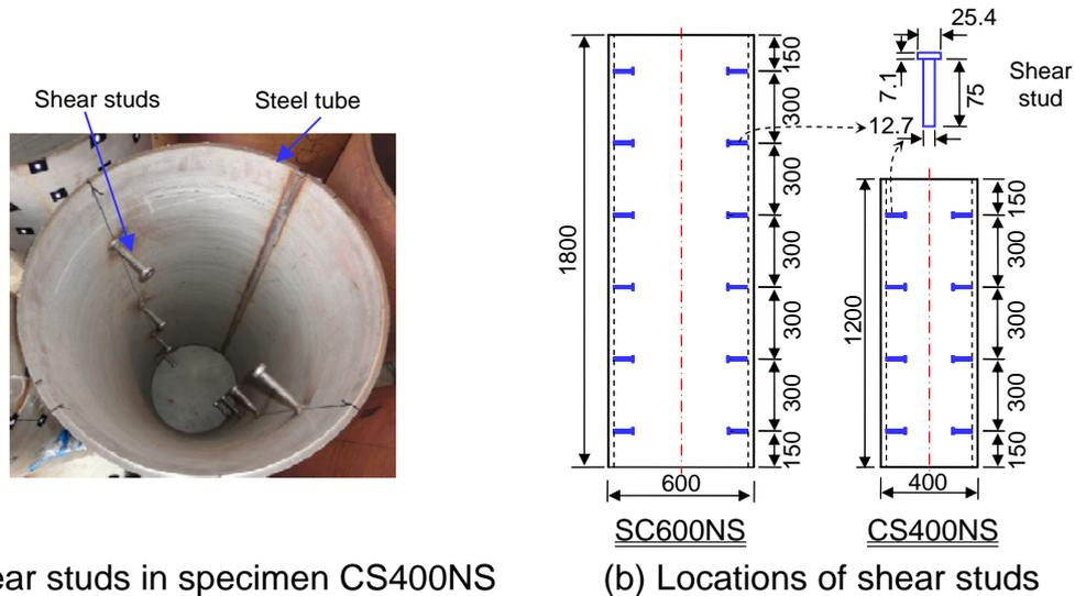
Fig. 1 Specimens with shear studs (unit: mm)
