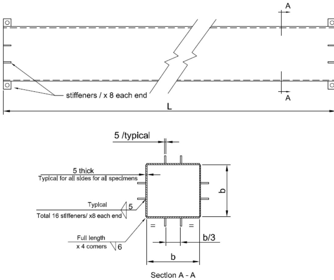
Fig. 1 Dimensions of the test specimens.
