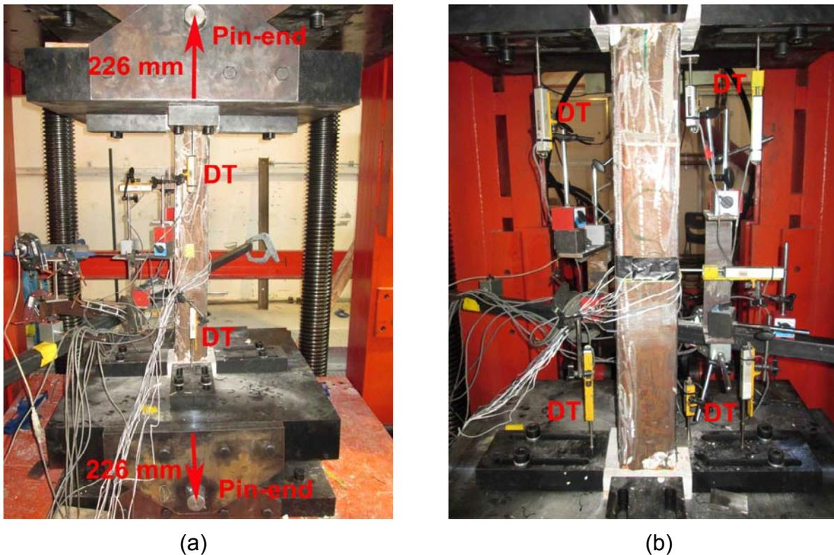
Fig. 2 Test procedures and locations of displacement transducers (DTs): (a) Front view of the test setup and (b) Side view of the test setup.
