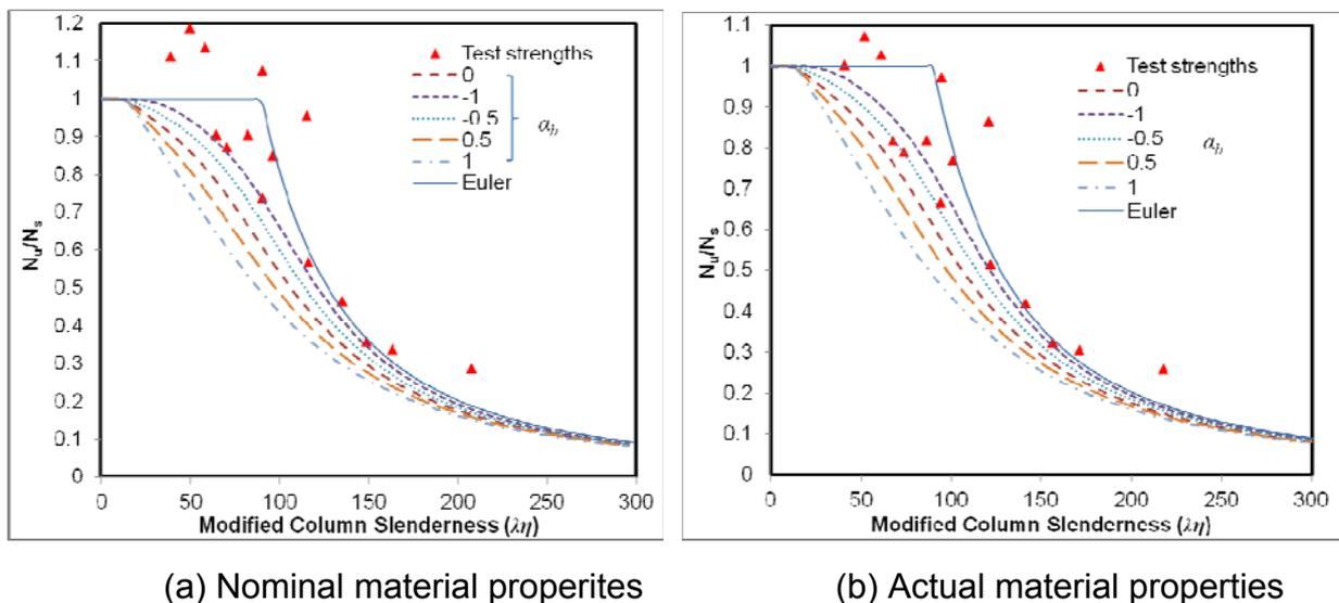
Fig. 5 Comparison of column curves of AS5100.6 and non dimensional test strengths.
