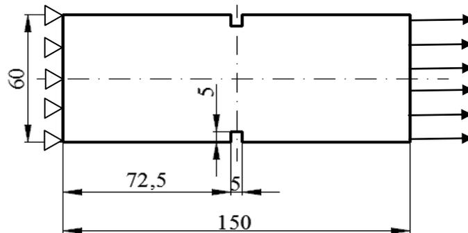
Fig. 4. Setup for the second test (dimensions in mm)
