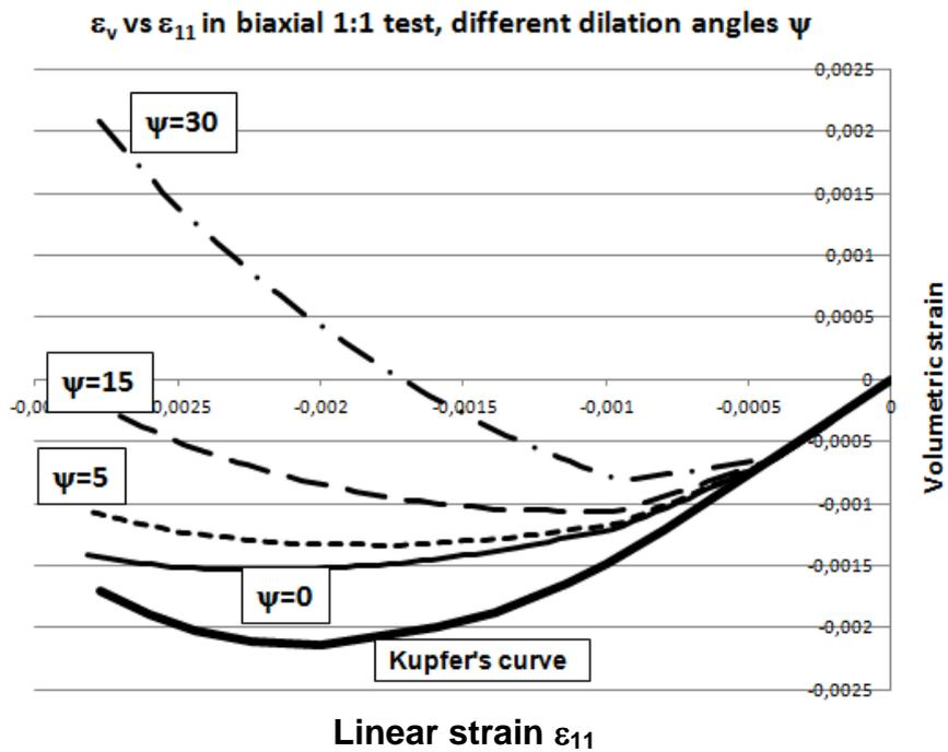
Fig. 15. Volumetric strain in biaxial 1:1 compression test
