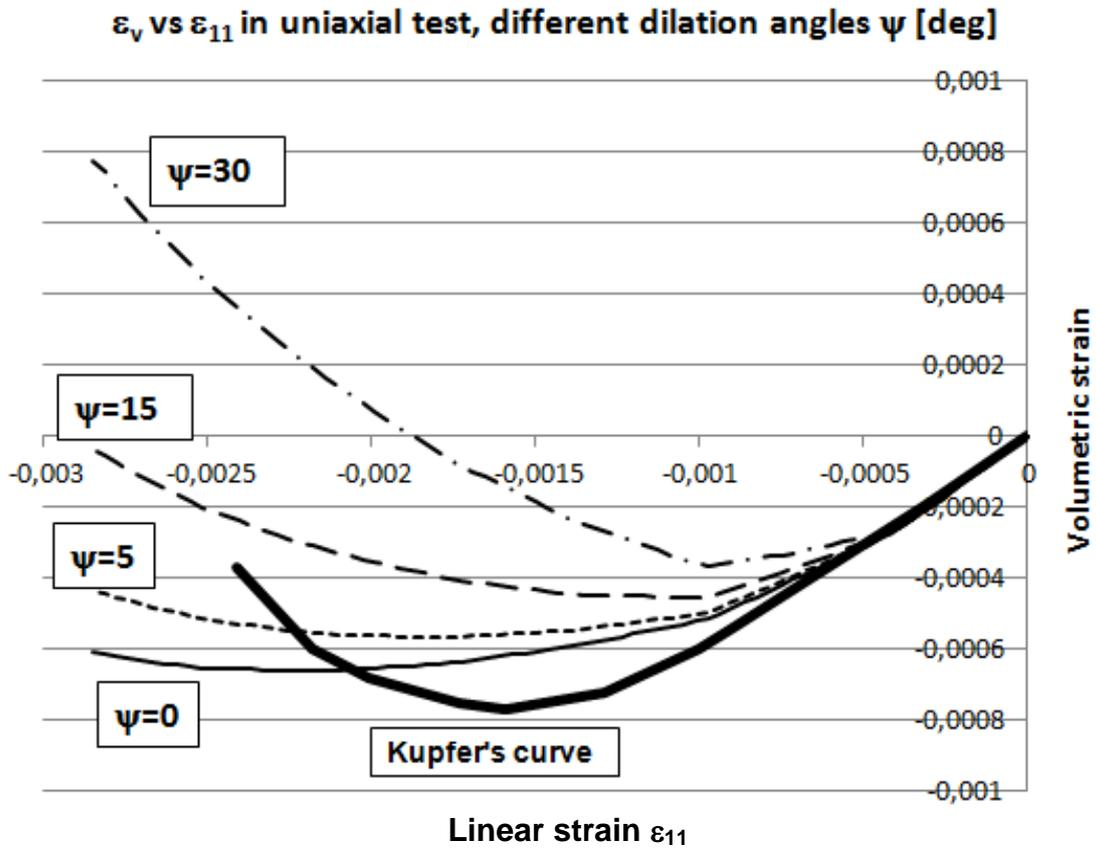
Fig. 14. Volumetric strain in uniaxial compression test
