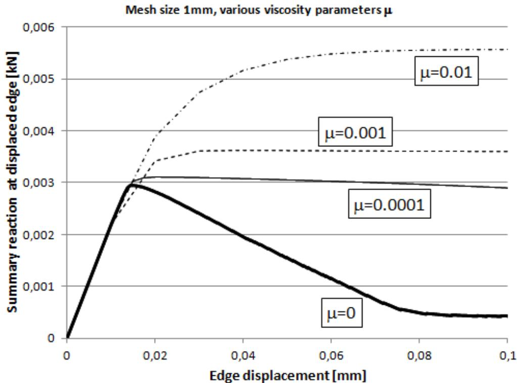
Fig. 13. Displacement vs summary reaction for 1mm mesh size
