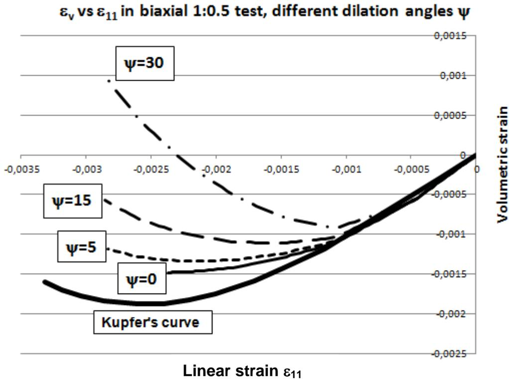
Fig. 16. Volumetric strain in biaxial 1:0.5 compression test
