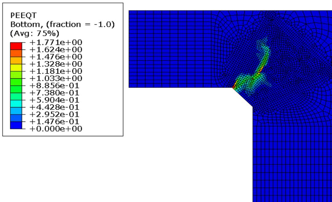
Fig. 2. Equivalent plastic strains in tension
