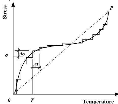
Fig. 1. Temperature-stress discretizing load path.
