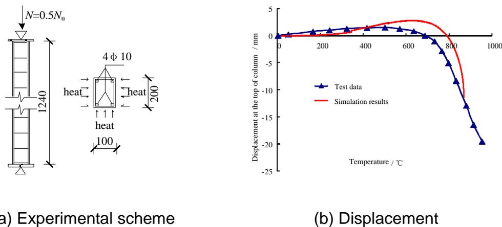
Fig. 4. RC column exposed to three-side fire.
