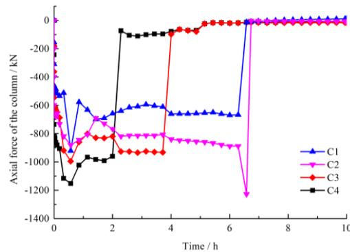
Fig. 9. The axial force of the frame columns subjected to fire.
