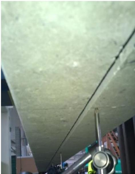
Fig.2 Slit Cast in Bottom of Beam
