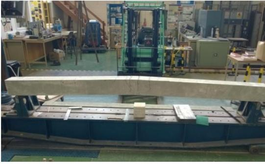
Fig.4 Residual Damage to Control Beam
