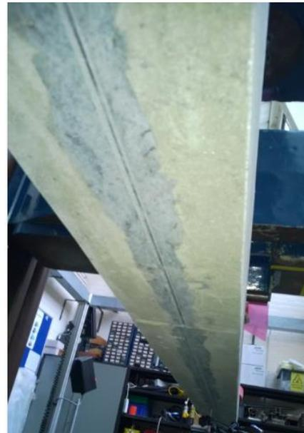
Fig.3 CFRP Bonded inside the Slit
