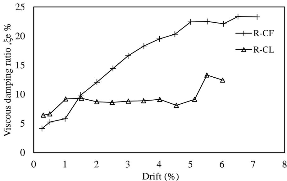
Fig. 10- Viscous damping ratio versus column drift of R-CF and R-CL columns
