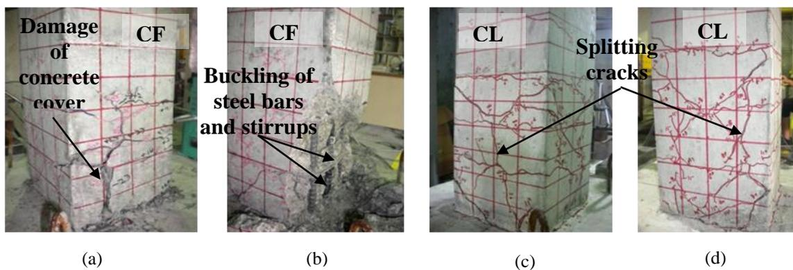
Fig. 3- Final failure pattern of (a & b) CF column and (c & d) CL column
