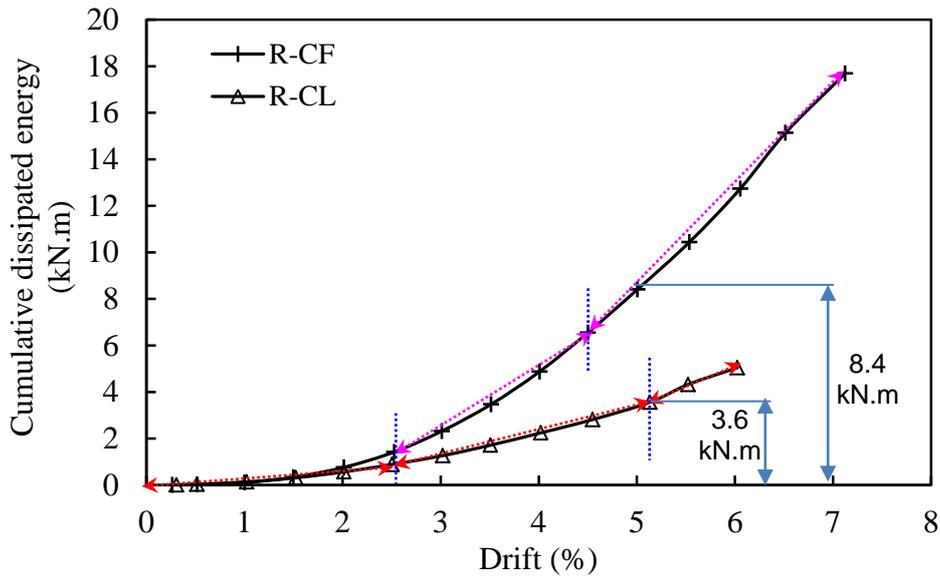
Fig. 9- Cumulative dissipated energy versus column drift of R-CF and R-CL columns
