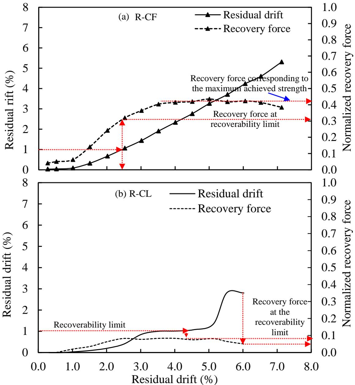
Fig. 8- Load-versus drift response of CL and CF after repair (a) R-CL and (b) R-CF
