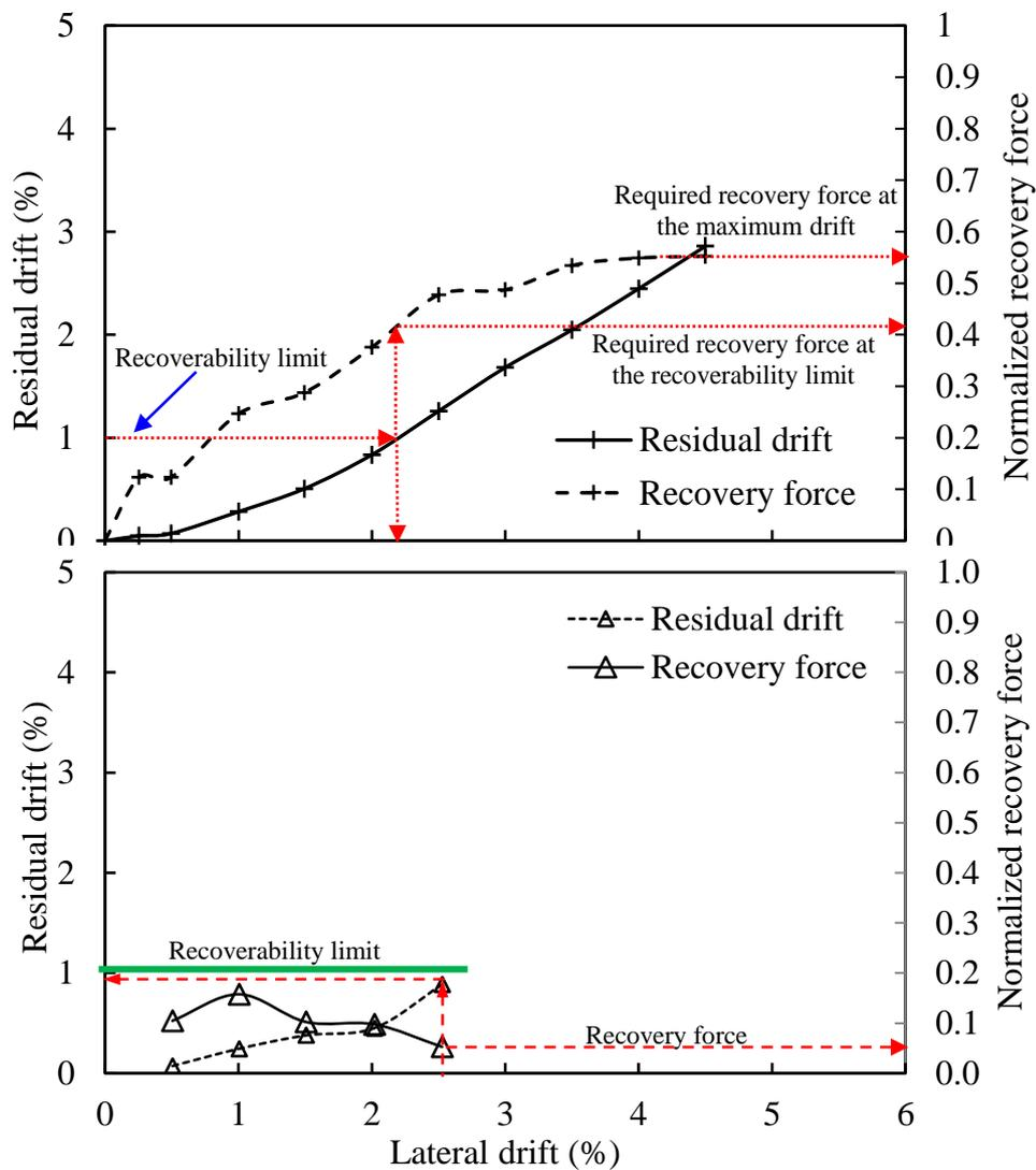
Fig. 4 Column lateral load versus residual drift and the normalized recovery force of (a) CF column and (b) CL column
