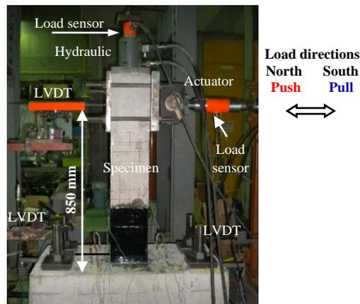
Fig. 1- Specimen during testing
