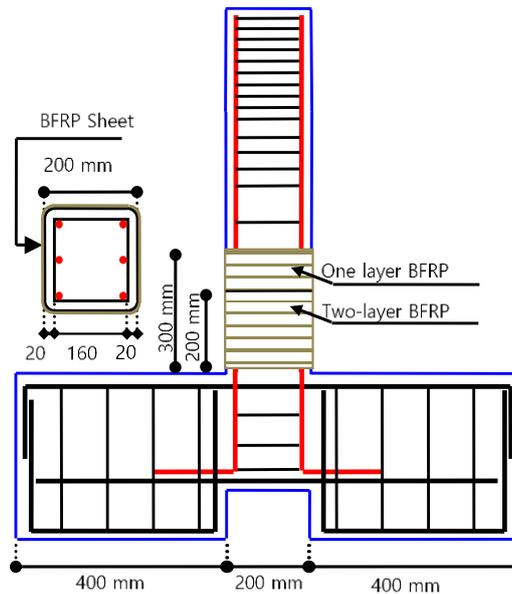
Fig. 6- Details of BFRP repaired columns R-CL and R-CL
