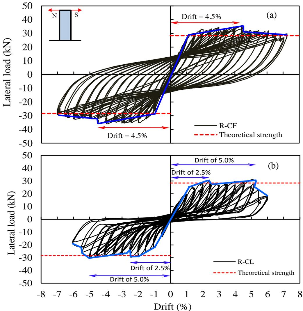
Fig. 7- Load-versus drift response of CL and CF after repair (a) R-CL and (b) R-CF
