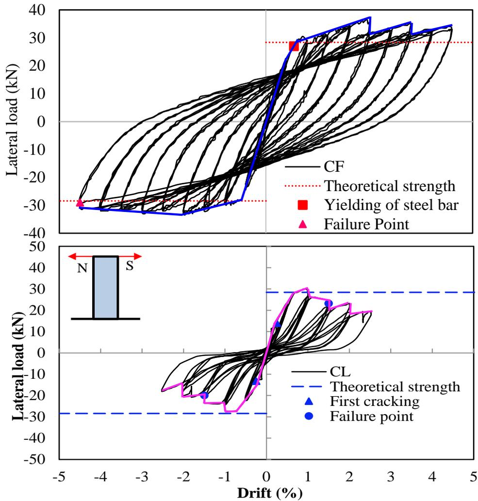
Fig. 2- Load-versus drift response of CL and CF
