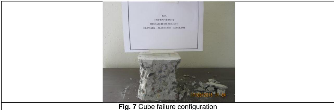
**Fig. 7** Cube failure configuration
