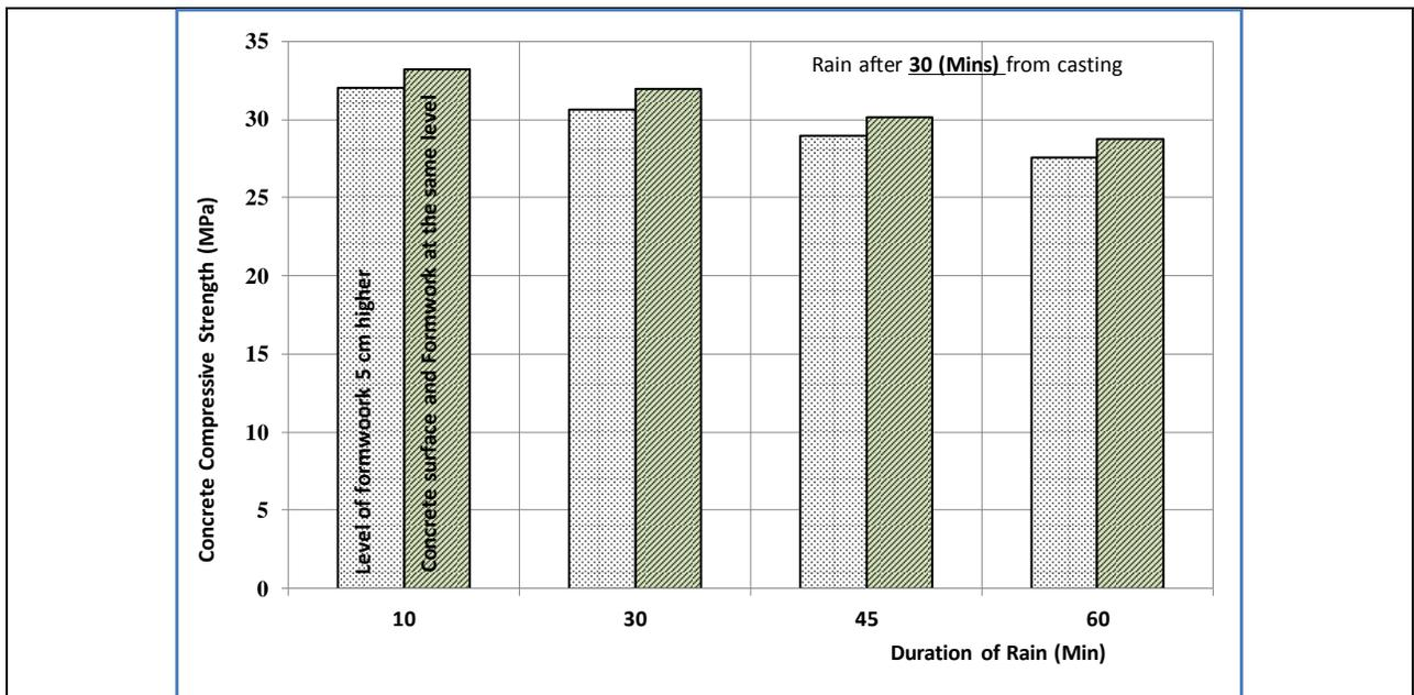
**Fig. 9** Comparison between concrete samples with different level of formwork from concrete surface and subjected to rainfall after 30 minutes from casting
