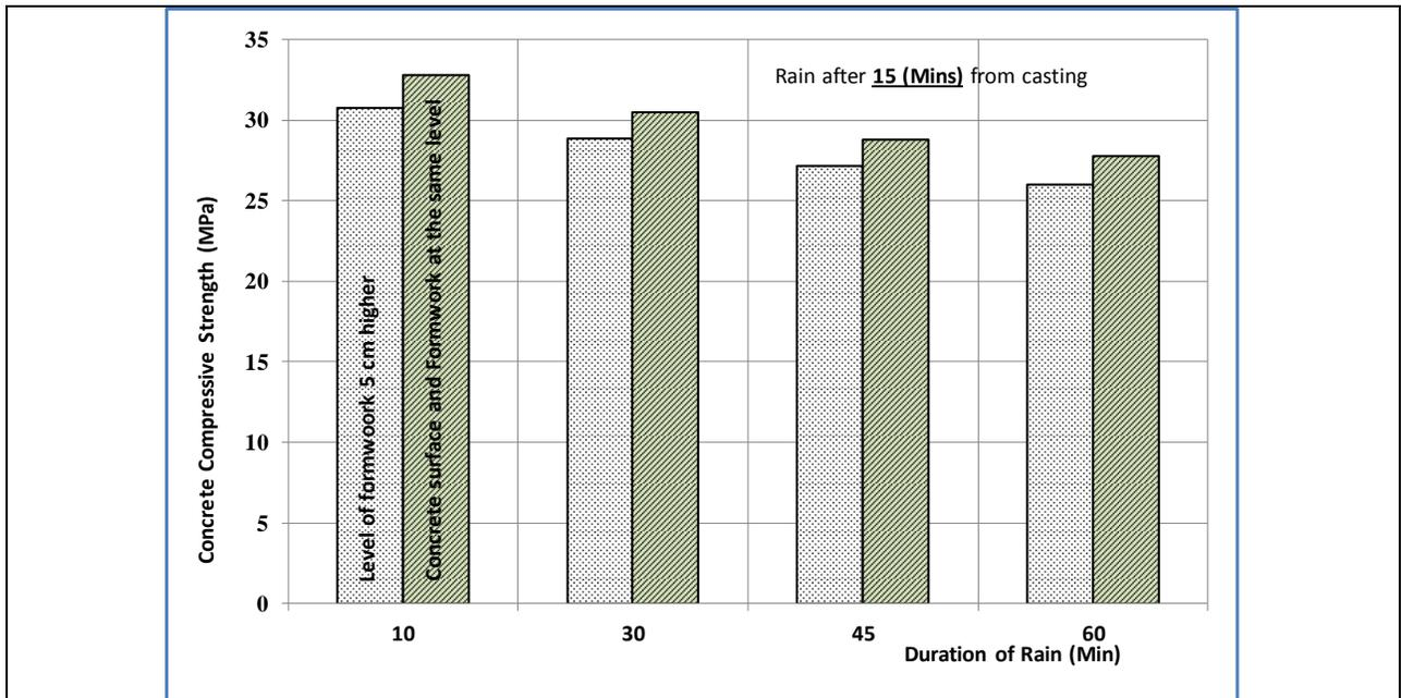
**Fig. 8** Comparison between concrete samples with different level of formwork from concrete surface and subjected to rainfall after 15 minutes from casting
