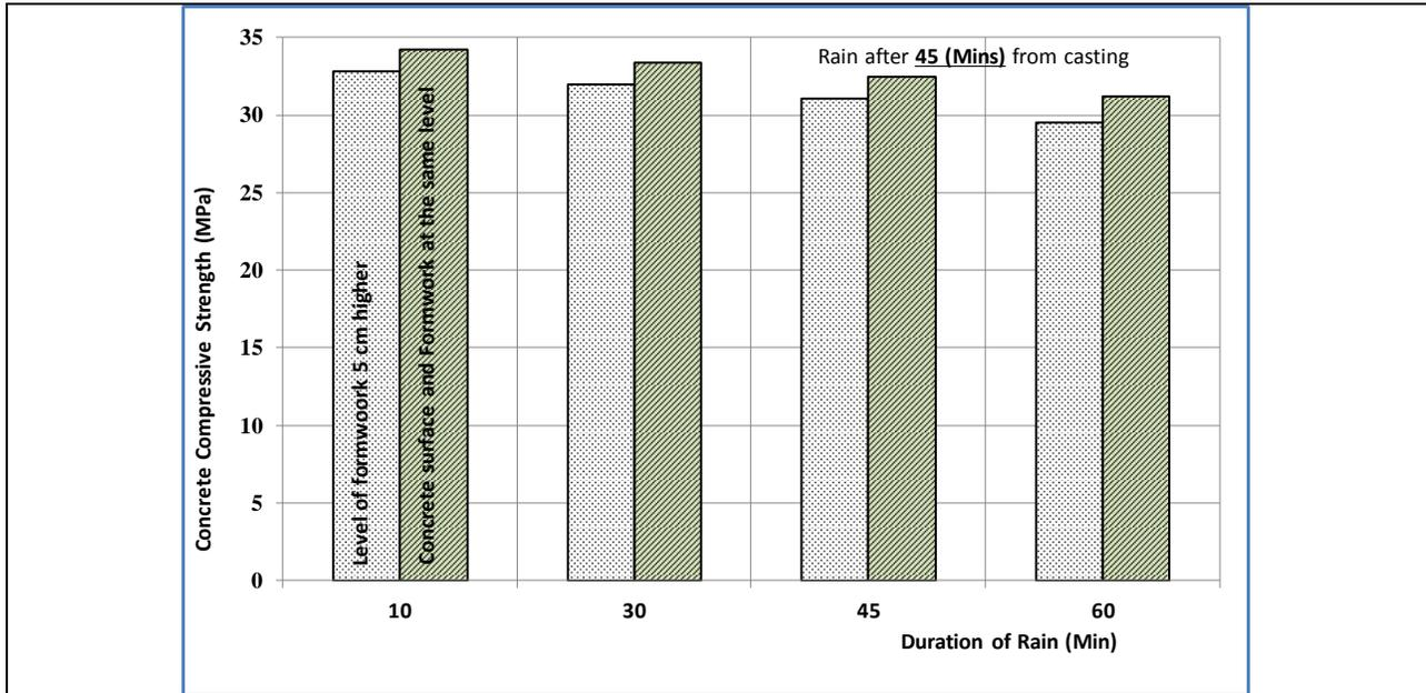
**Fig. 10** Comparison between concrete samples with different level of formwork from concrete surface and subjected to rainfall after 45 minutes from casting
