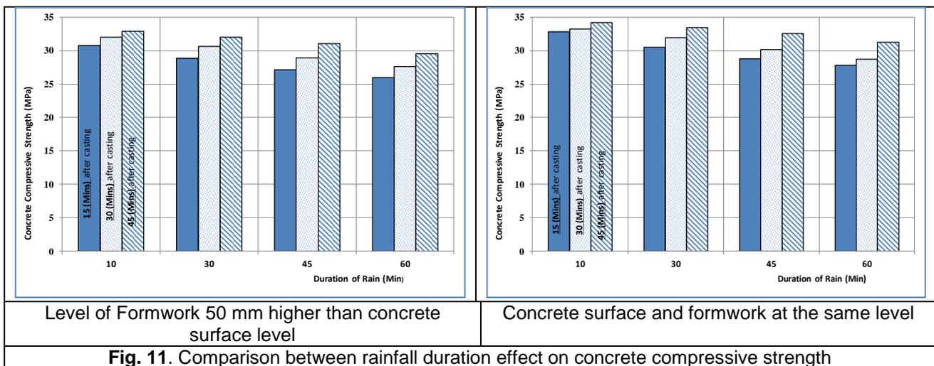
**Fig. 11.** Comparison between rainfall duration effect on concrete compressive strength
