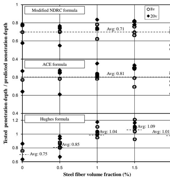
Fig. 1 Penetration depth to predict depth ratios according to steel fiber volume fraction
