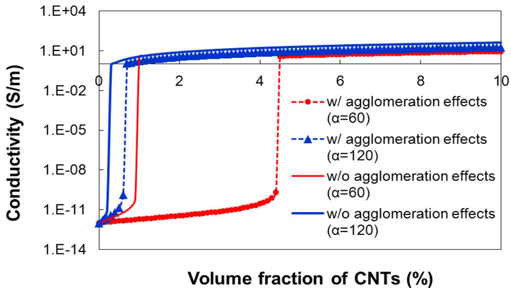
Figure 1. The predicted electrical conductivity of the nanocomposites with respect to the aspect ratio ( $\alpha$ ) and agglomeration of CNT
