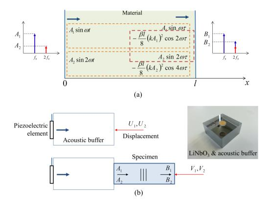
Fig. 1 Absolute second harmonic nonlinear parameter measurement, (a) Conceptual diagram for initial 2<sup>nd</sup> harmonic component, (b) Schematic diagram for initial 2<sup>nd</sup> harmonic component measurement.
