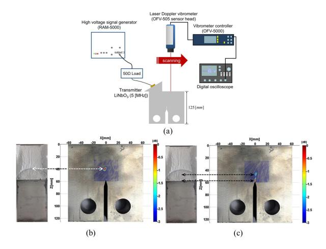
Fig. 2 Measurement system and imaging results, (a) Schematic diagram of experimental apparatus, Cross-section of the specimen with phased array images for (b) Sub-harmonic frequency (2.5 [MHz]) that is assumed to show closed part indicated by white arrow, (c) Fundamental frequency (5 [MHz]) that shows open part indicated by black arrows.
