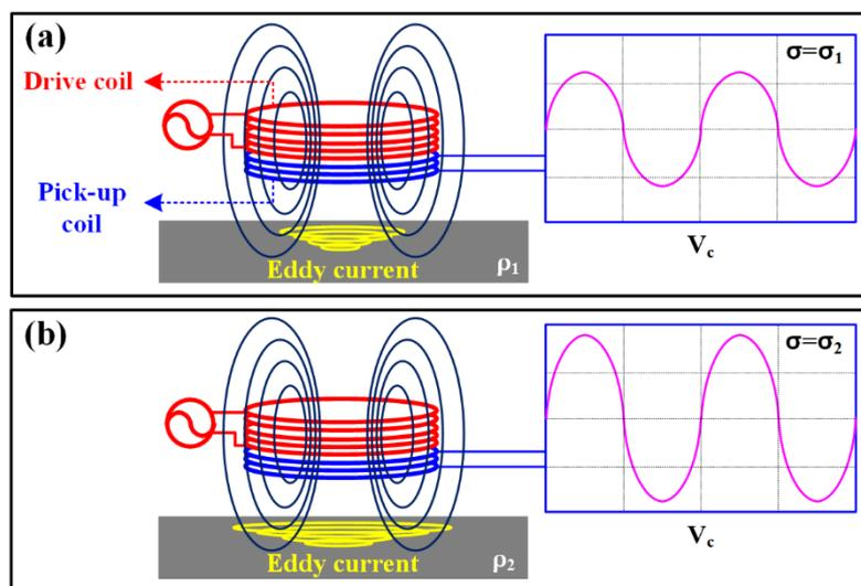
Fig. 1. Basic configuration of ECT to evaluate a target structure subjected to different stress conditions: (a)  $\sigma = \sigma_1$ , (b)  $\sigma = \sigma_2$
