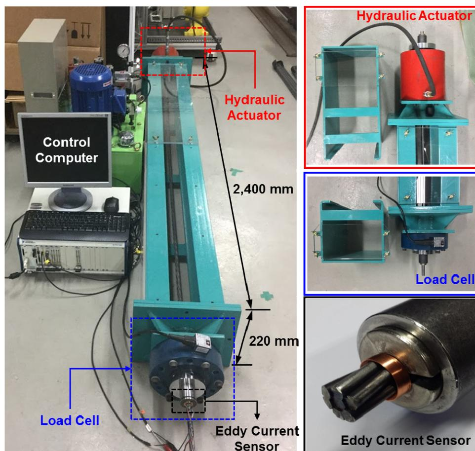
Fig. 5. Experimental setup of EC-TFI system using a cylinder-type ECS
