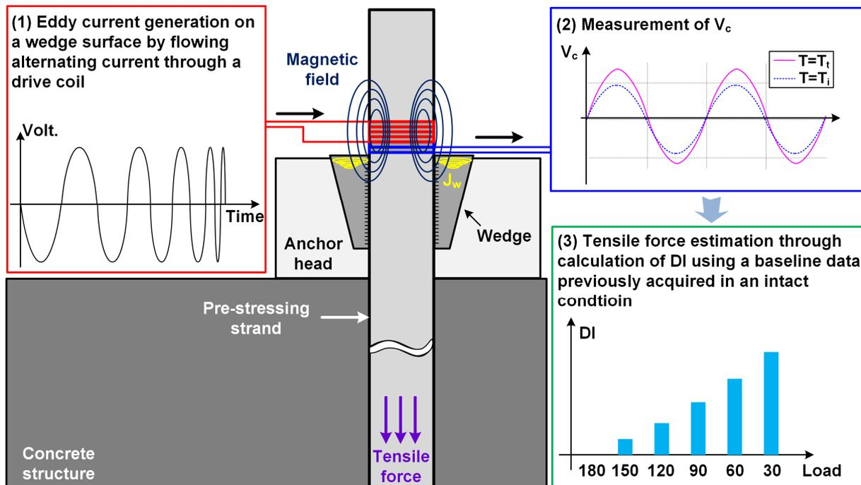
Fig. 3. Detailed working steps of the proposed EC-TFI
