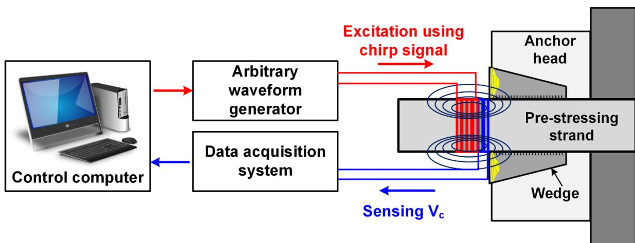
Fig. 4. Schematics of the developed EC-TFI system
