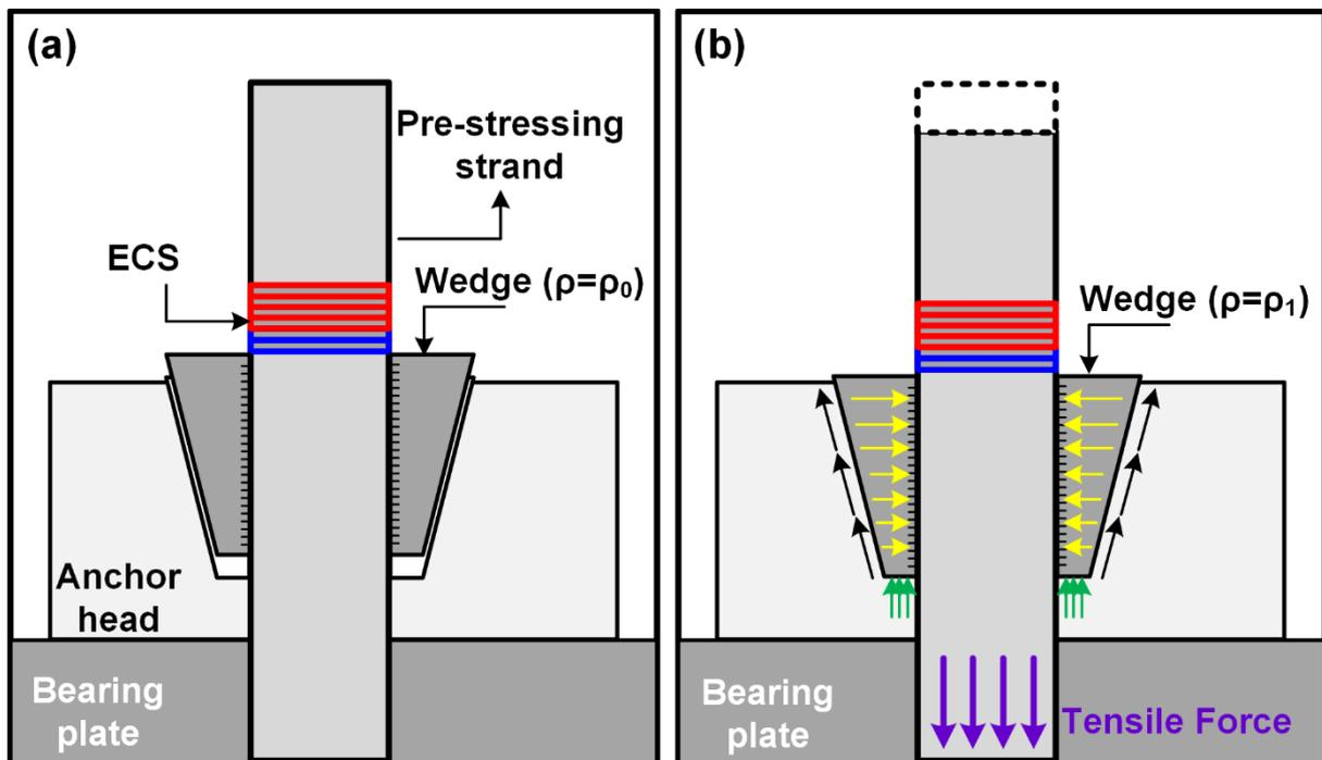
Fig. 2. Stress distribution of the exposed surface of a wedge:
