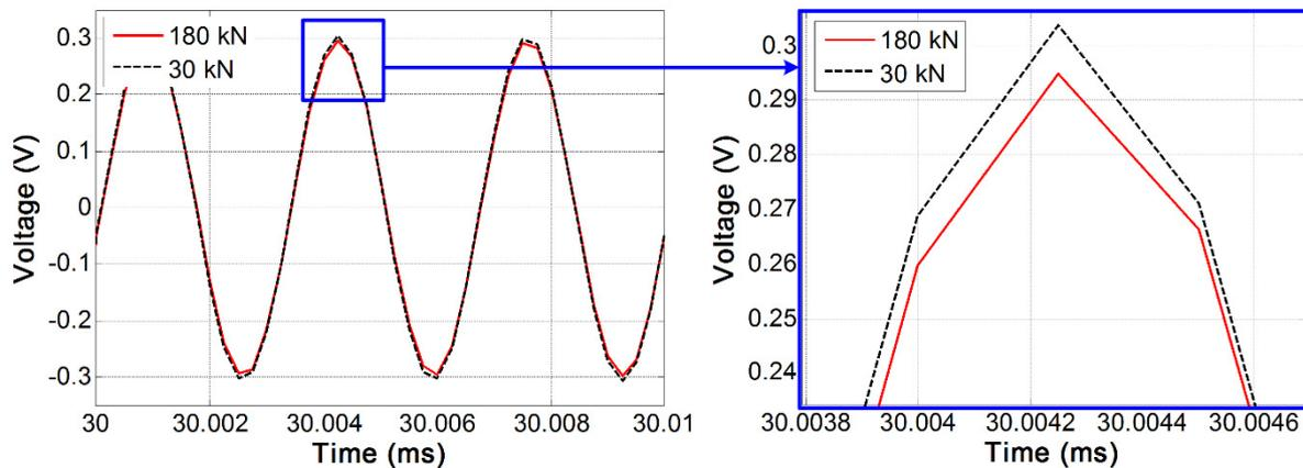
Fig. 7. Comparison the measured  $V_c$ 's under 180 kN and 30 kN which is expressed using red-solid line and black-dotted line, respectively.
