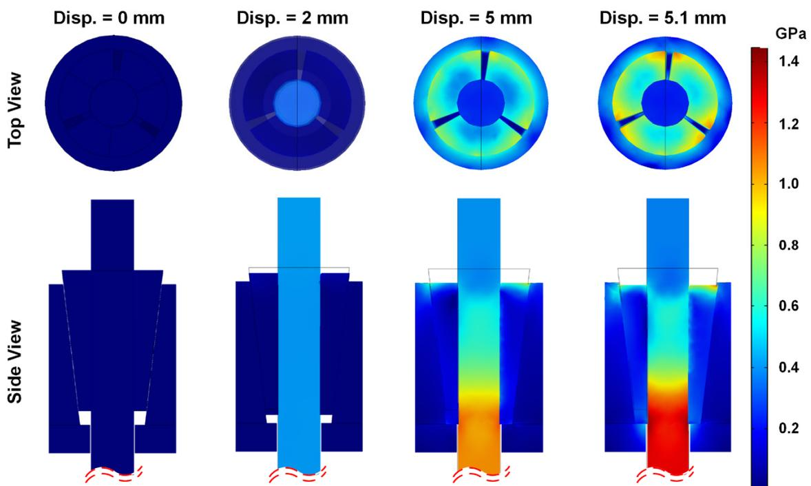
Fig. 6. Numerical simulation for stress distribution of a wedge holding a pre-stressing strand using finite element analysis
