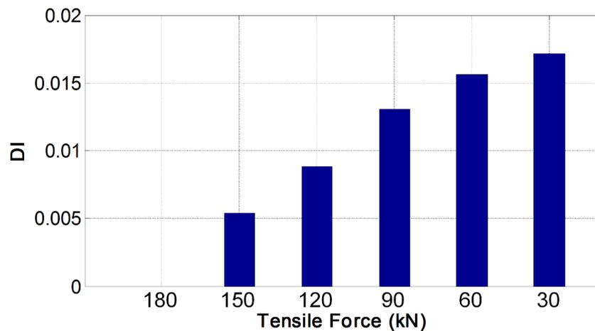
Fig. 8. DI comparison under 30 kN step-wise tensile force loss from an initial tensile force of 180 kN using a cylinder-type ECS
