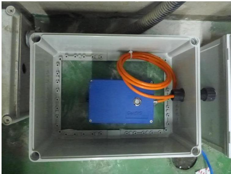
Fig. 10 Installation picture of the seismometer
