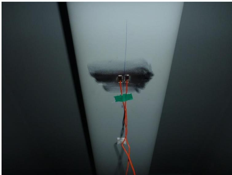
Fig. 11 Installation picture of foil-type strain gauges
