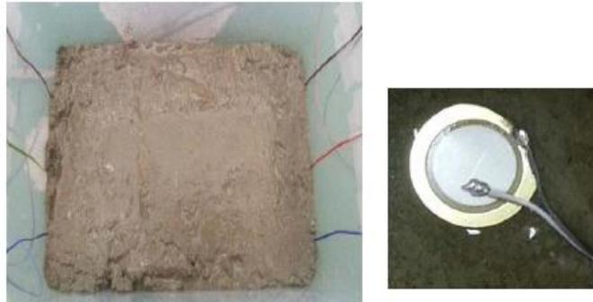
**Fig.1 Concrete cube and PZT transducer**
