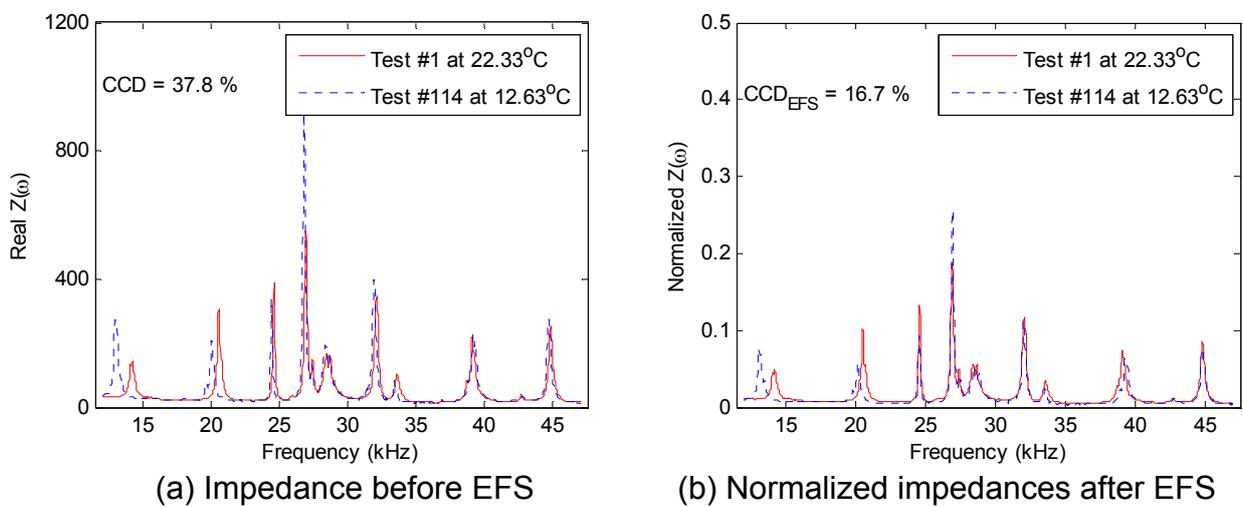
Fig. 11 Impedance signatures for frequency range 12-47 kHz measured from intact tendon-anchorage for two different temperatures: 22.3°C versus 12.63°C
