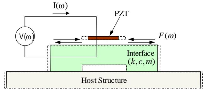
Fig. 2 PZT interface-structure model for SM impedance response
