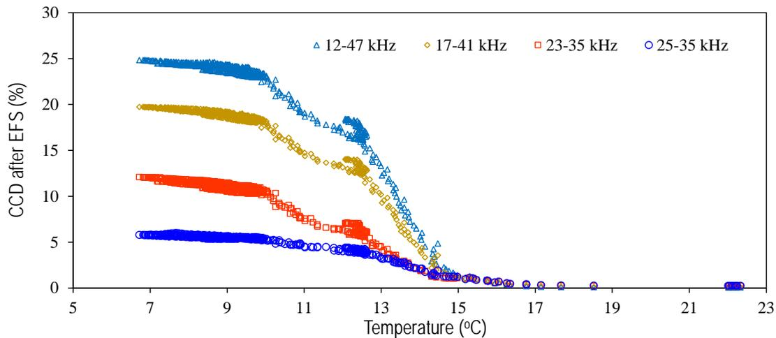
Fig. 14 CCD index after EFS for various frequency ranges of impedance signatures measured from intact tendon-anchorage for temperatures: 6.72°C ~ 22.33°C (Reference: Test #1 at 22.33°C)
