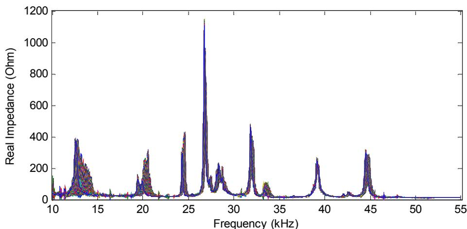
Fig. 9 Impedance signatures for frequency range 10-55 kHz measured from intact tendon-anchorage for temperatures:  $6.72^{\circ}\text{C} \sim 22.33^{\circ}\text{C}$
