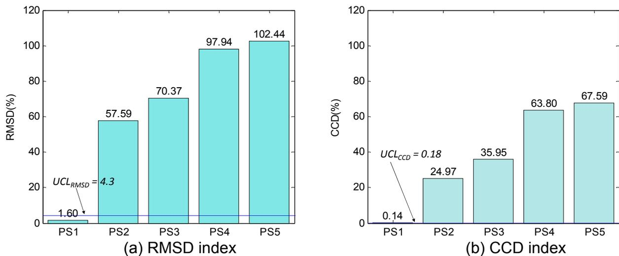
Fig. 8 Prestress force-loss monitoring results under constant temperatures
