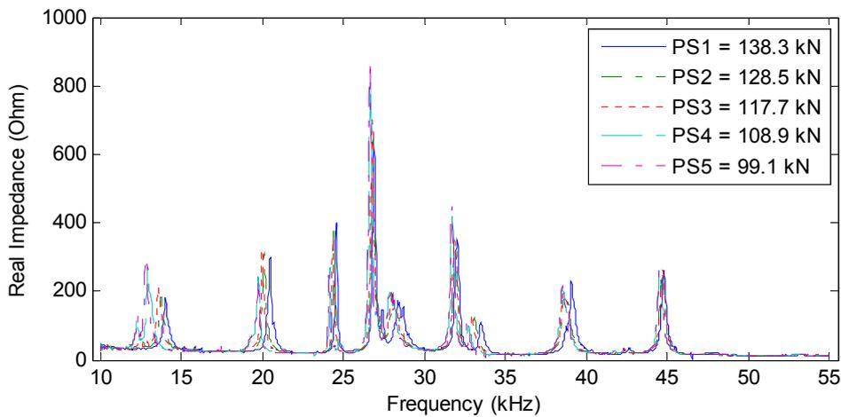
Fig. 7 Impedance signatures of PZT interface under various prestress forces
