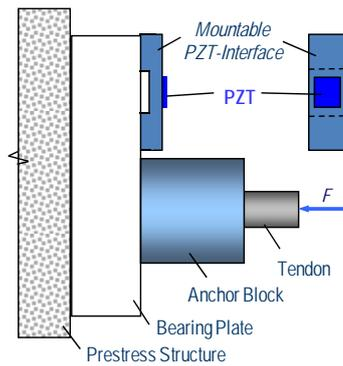
Fig. 1 Prestressed tendon-anchorage system with a mountable PZT interface
