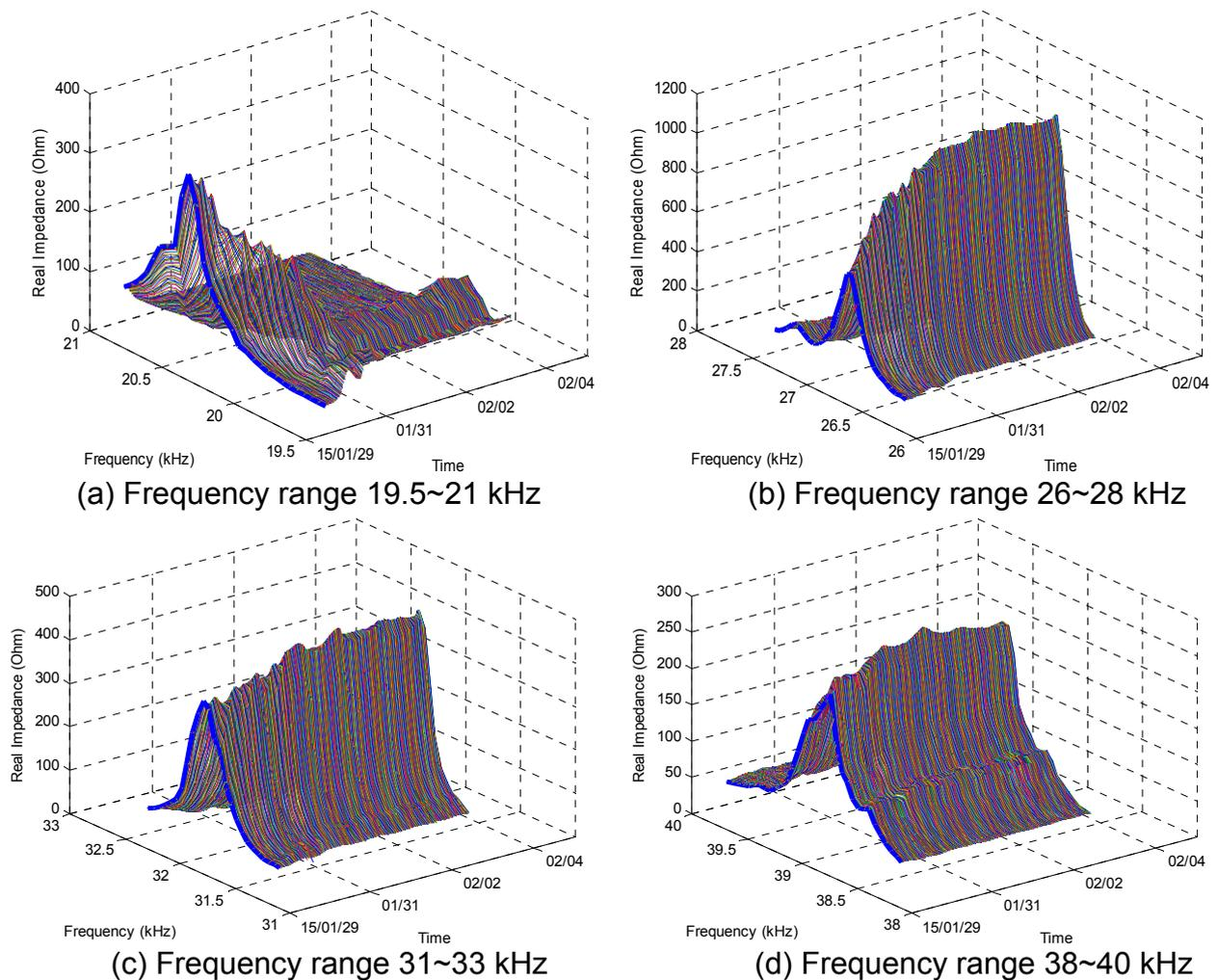
Fig. 10 Time history of resonant peaks of impedance signatures measured from intact tendon-anchorage for temperatures: 6.72°C ~ 22.33°C
