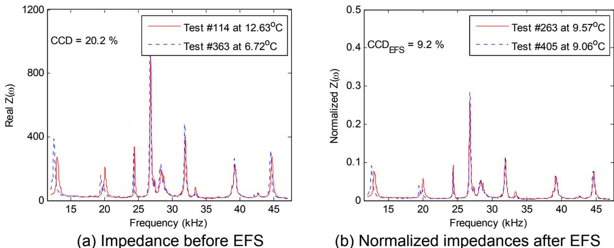
Fig. 12 Impedance signatures for frequency range 12-47 kHz measured from intact tendon-anchorage for two temperatures: 12.63°C versus 6.72°C
