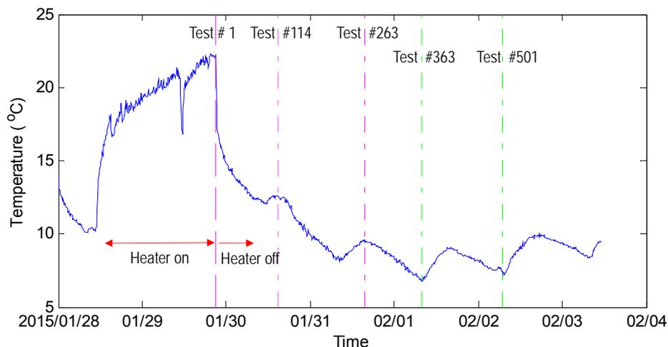
Fig. 5 Temperature history of temperature variation simulated in laboratory
