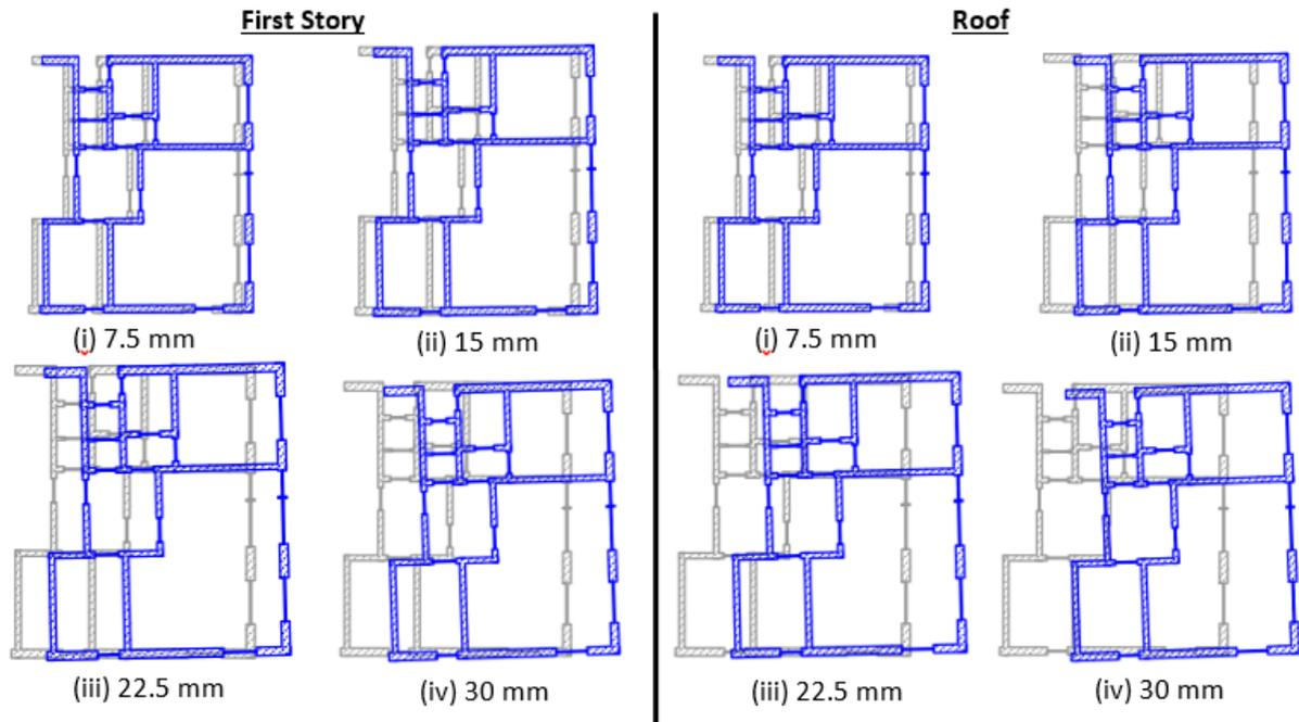
**Figure 13.** Plan Deflections at Different Roof Displacements for Each Story Level
