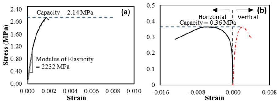
**Figure 9.** (a) Compressive Stress-Strain Curves and (b) Diagonal Tension Stress-Strain Curves
