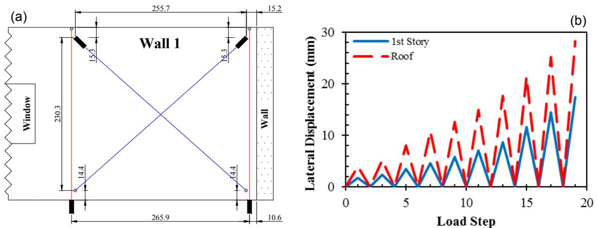
**Figure 7.** (a) The installed LVDT's for a Representative Wall and (b) Control Displacements applied to Each Story (All units are in cm.)
