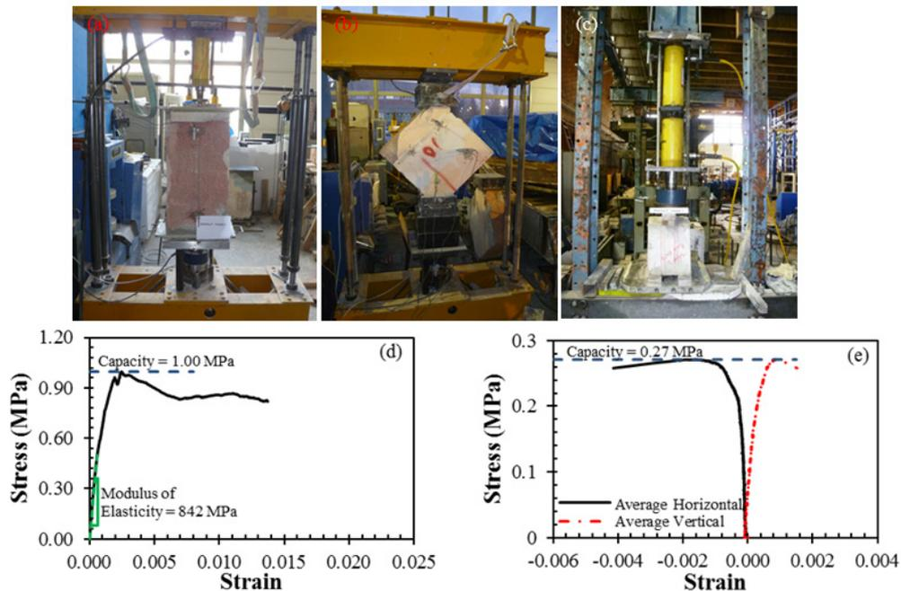
**Figure 2.** Material Test Setups and Test Results : (a) Compression Test Setup , (b) Diagonal Tension Test Setup, (c) Triplet Test Setup, (d) Compressive Stress-Strain Curve and (e) Diagonal Tension Stress-Strain Curves
