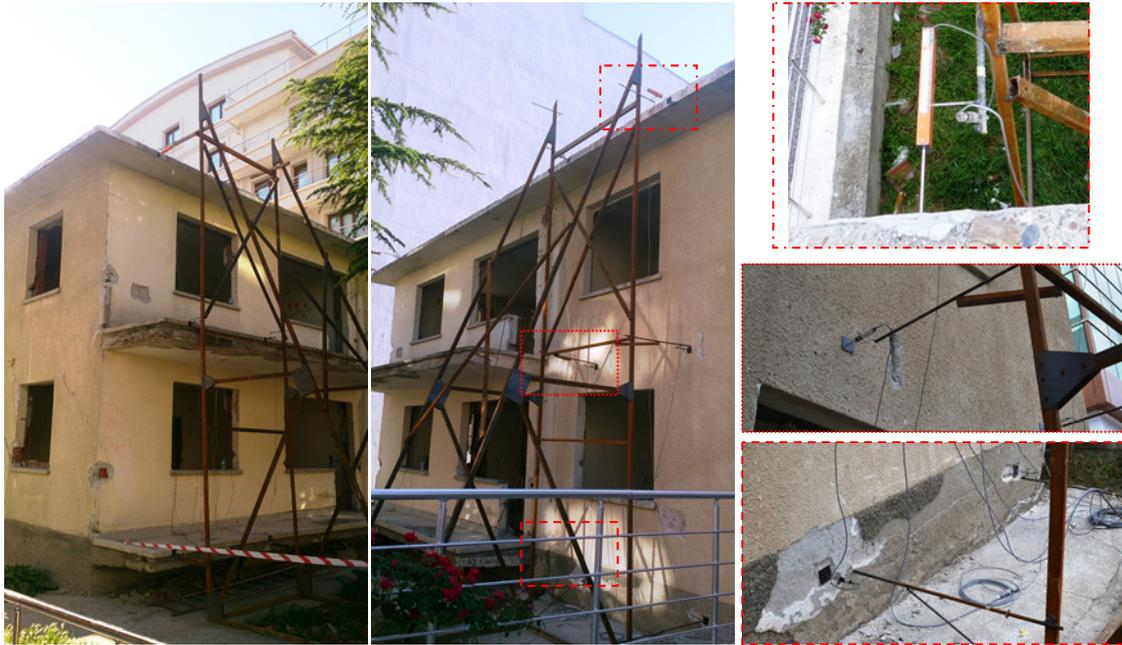
**Figure 6.** Photos of LVDT's installed at Each Story Level
