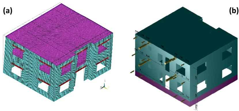
**Figure 11.** (a) Finite element model and (b) first mode shape
