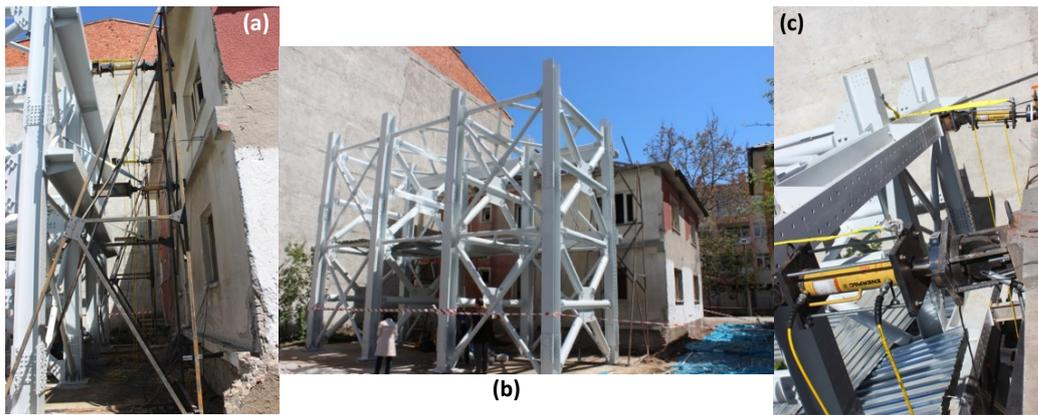
**Figure 10.** (a) Side view of LVDT's and hydraulic pistons, (b) photo of steel frame and (c) photos of hydraulic pistons at the second story
