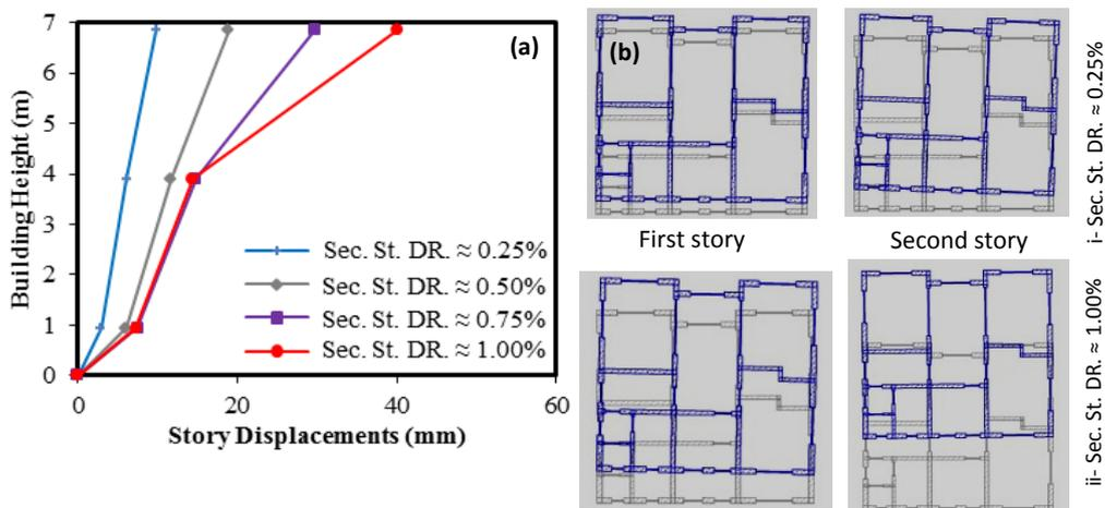
**Figure 16.** (a) Deformation profile at different drift ratio levels of the second story and (b) plan deflection of first and second stories at a drift ratio of (row i) 0.25% and (row ii) 1.00%
