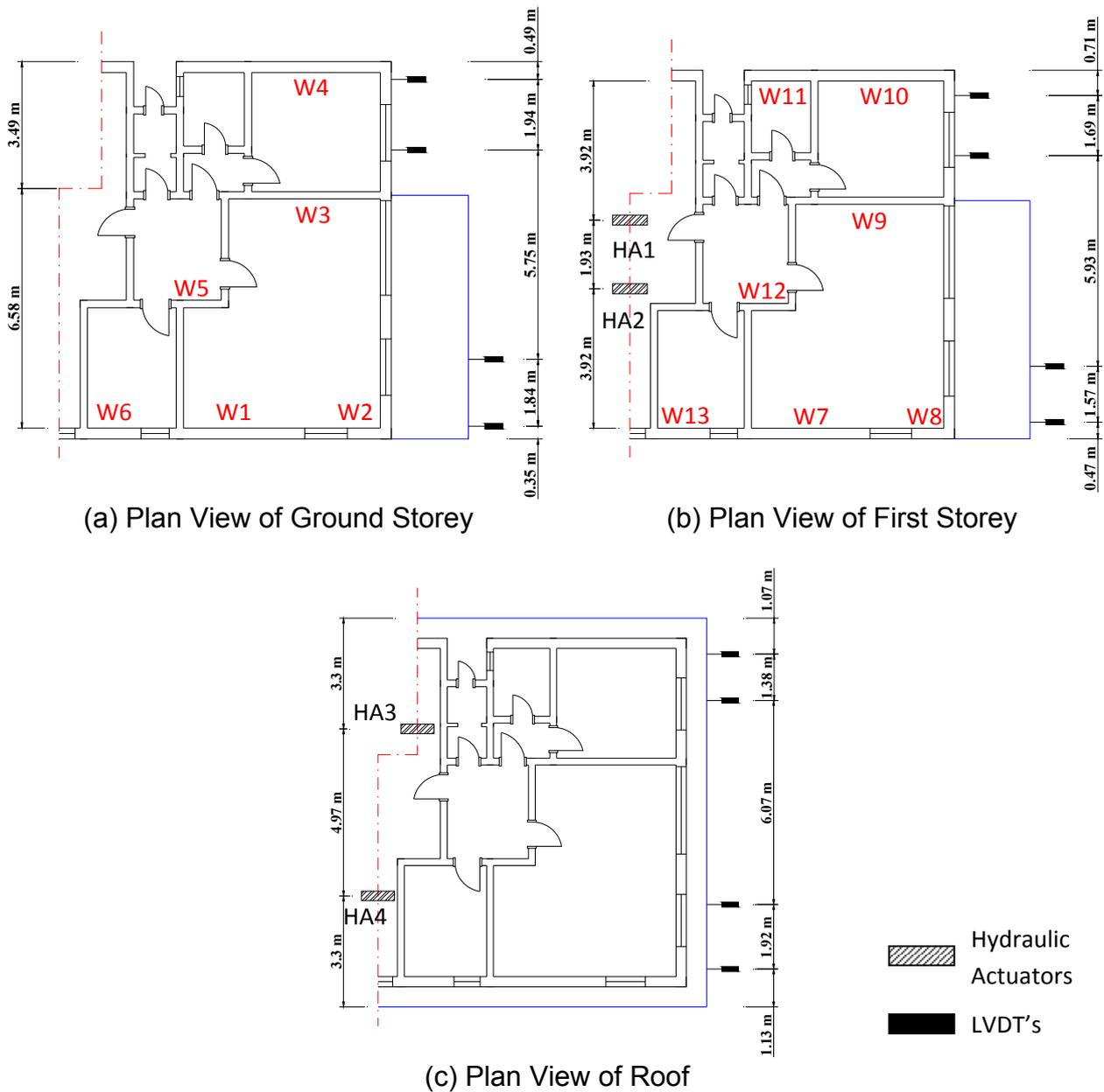
**Figure 4.** Locations of Hydraulic Actuators and LVDT's
