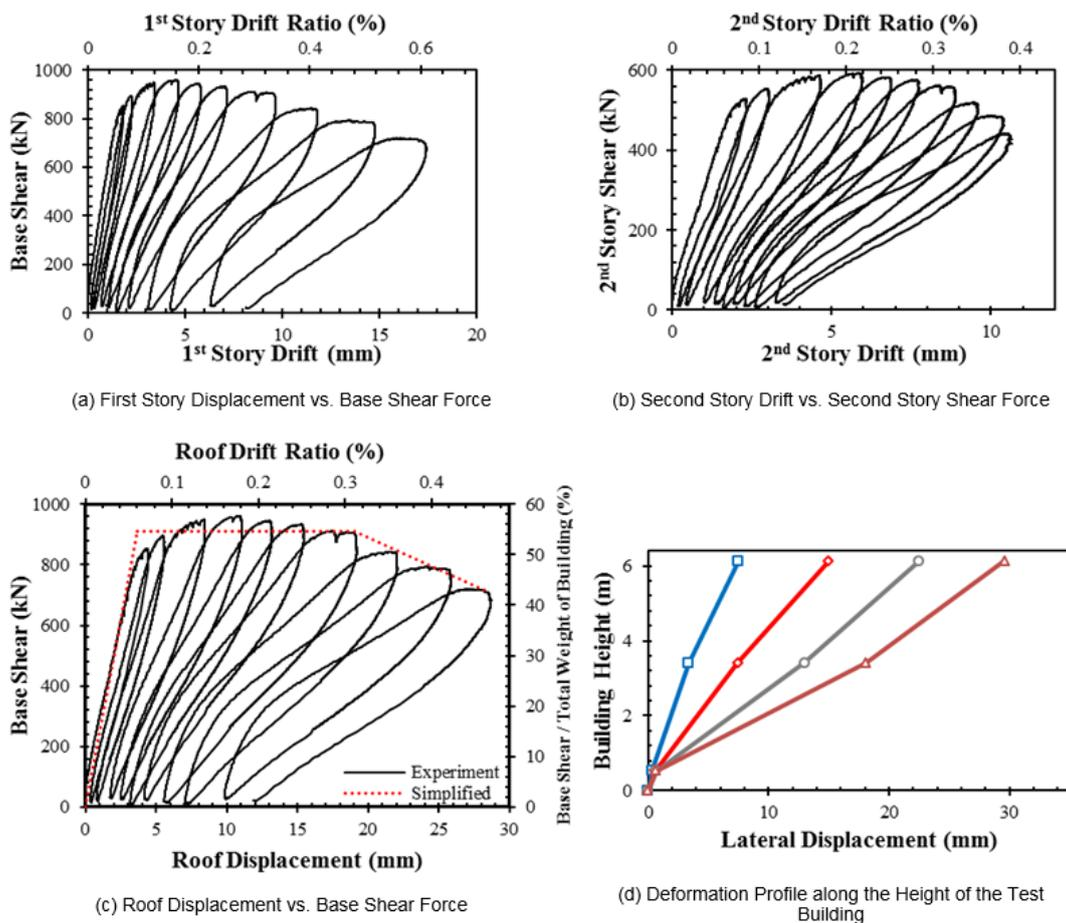
**Figure 12.** Recorded Load – Deformation Responses
