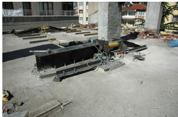
(b) Hydraulic Actuators at the Roof
