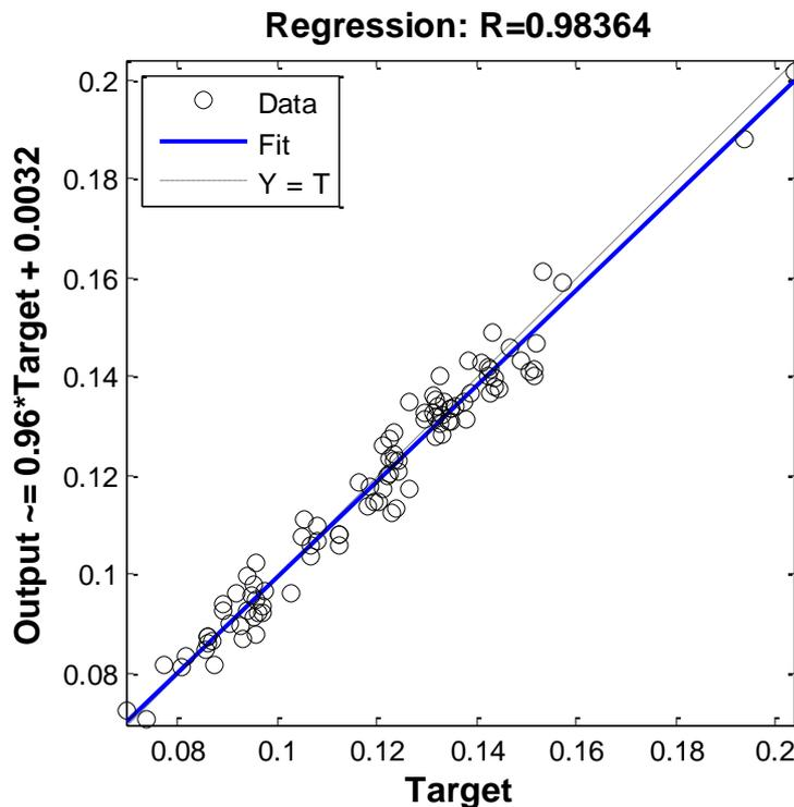
Fig. 3 Regression analysis of the surrogate model output on the output derived from the fourth-order Runge-Kutta method (i.e., the time marching method)
