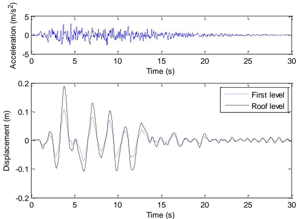
Fig. 1 A synthetic seismic horizontal ground acceleration record (the upper subfigure) and the resulting horizontal displacement response of the two-story hysteretic RC frame (the lower subfigure)
