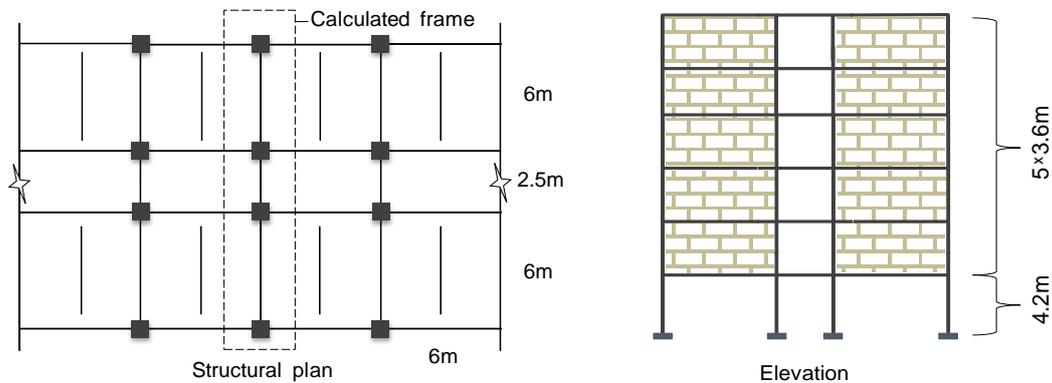
Fig. 3. Structural configuration.
