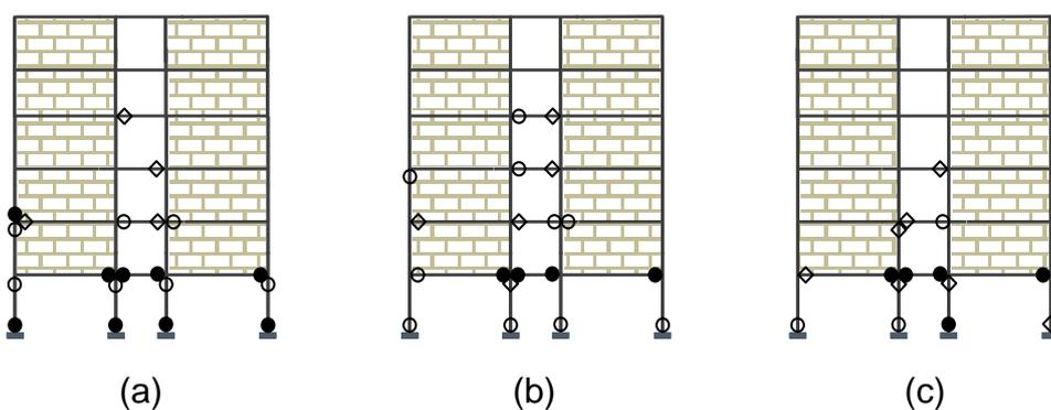
Fig. 14. The plasticity development of FRAME2 (a)  $K_{S,2}/K_{S,1}=2.95$ , (b)  $K_{S,2}/K_{S,1}=2.56$ , (c)  $K_{S,2}/K_{S,1}=2.54$ .
