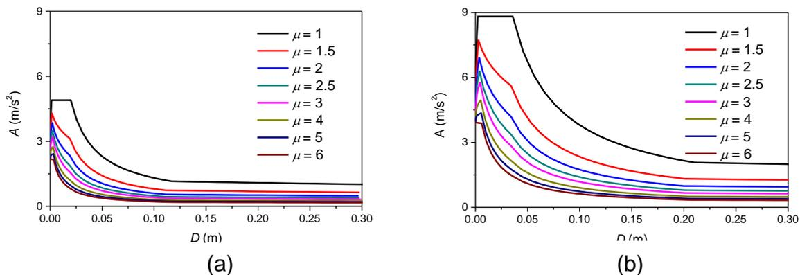
Fig. 4. Demand curves derived by design spectrum (a) For FRAME1, (b) For FRAME2.
