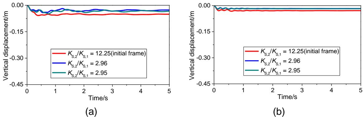
Fig. 17. Displacement time-history of FRAME1 with (a) the external column removed and (b) the external column removed after seismic strengthening.
