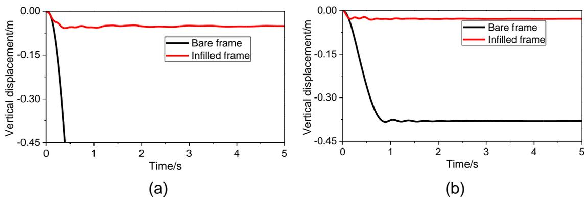
Fig. 11. Displacement time-history of FRAME1 with (a) the external column removed and (b) the external column removed.
