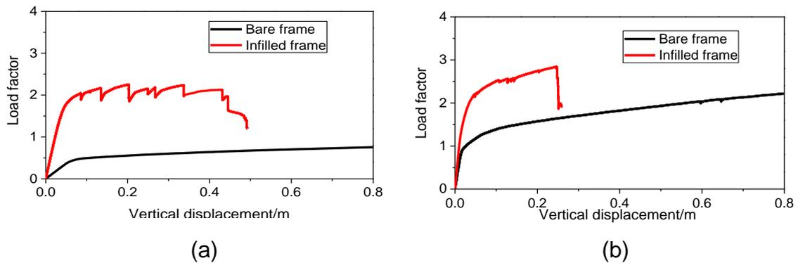
Fig. 10. Pushdown curves of FRAME2 with (a) the external column removed and (b) the external column removed.
