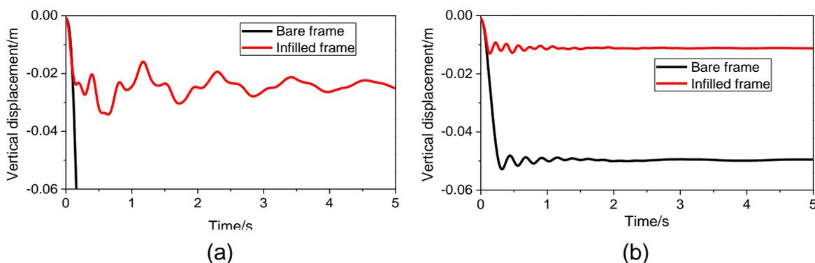
Fig. 12. Displacement time-history of FRAME2 with (a) the external column removed and (b) the external column removed.
