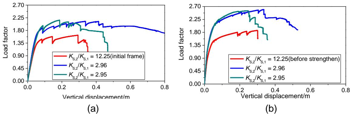
Fig. 15. Pushdown curves of FRAME1 with (a) the external column removed and (b) the external column removed after seismic strengthening.
