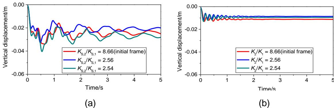
Fig. 18. Displacement time-history of FRAME2 with (a) the external column removed and (b) the external column removed after seismic strengthening.
