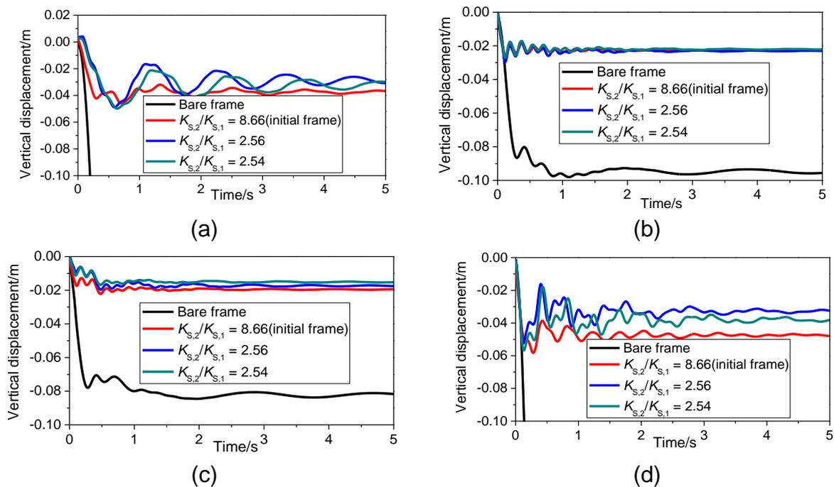
Fig. 20. Displacement time-history of FRAME2 with the earthquake-induced damage (a) Column A removed, (b) Column B removed, (c) Column C removed, (d) Column D removed.
