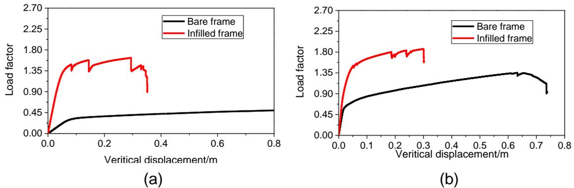
Fig. 9. Pushdown curves of FRAME1 with (a) the external column removed and (b) the external column removed.
