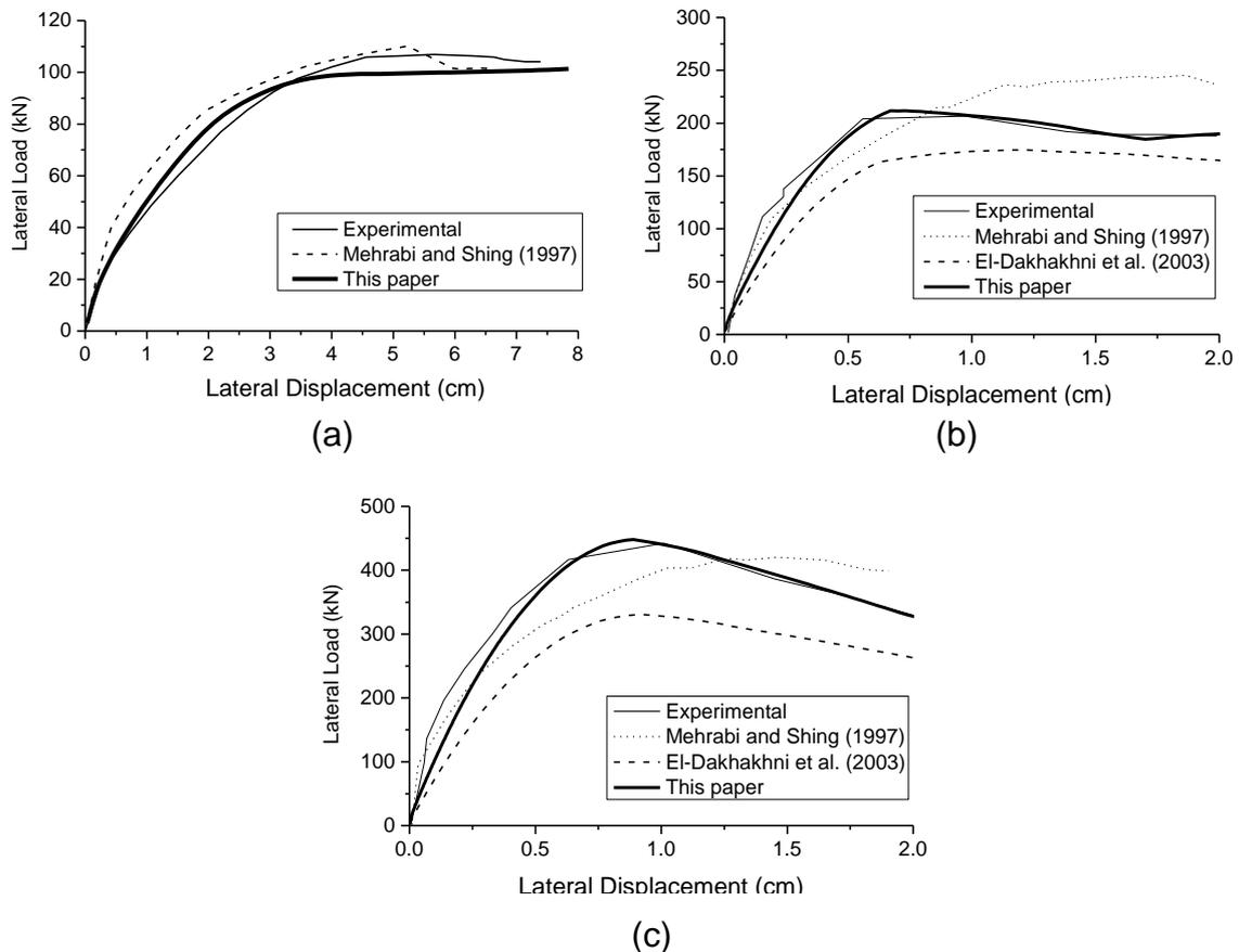
Fig. 2. Lateral load-displacement curves for (a) specimen 1, (b) specimen 6, and (c) specimen 7 in Mehrabi and Shing (1997) test.
