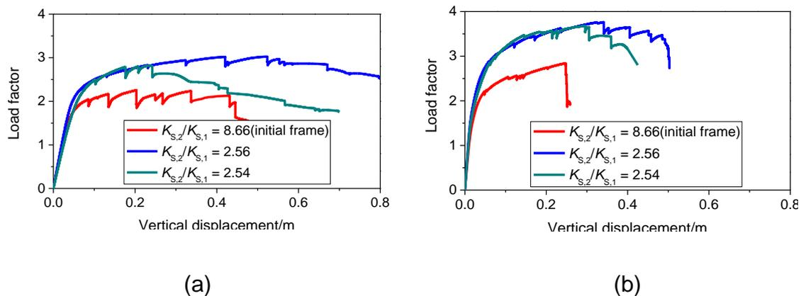
Fig. 16. Pushdown curves of FRAME2 with (a) the external column removed and (b) the external column removed after seismic strengthening.
