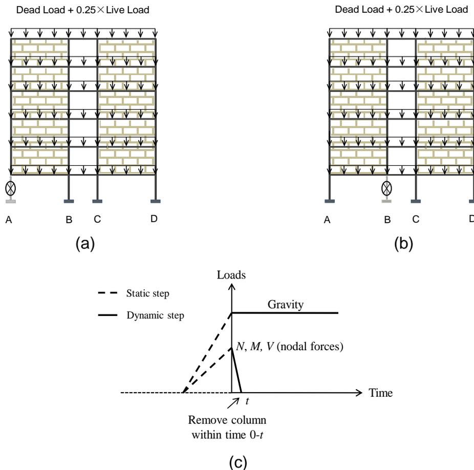
Fig. 8. Applied loads in static and dynamic analyses (a) With external column removed, (b) With internal column removed, (c) Dynamic analysis.
