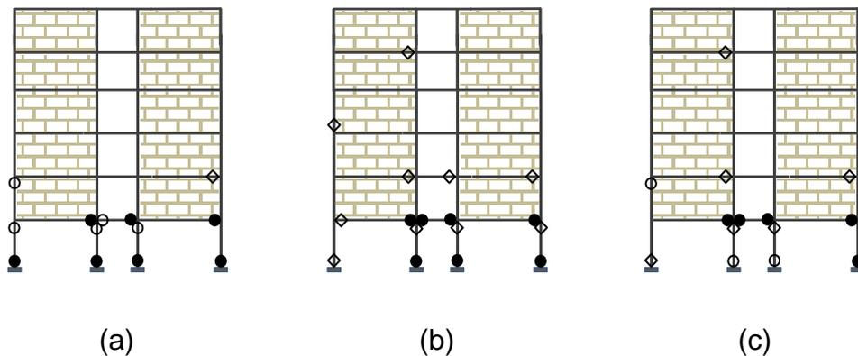
Fig. 13. The plasticity development of FRAME1 (a)  $K_{S,2}/K_{S,1}=3.33$ , (b)  $K_{S,2}/K_{S,1}=2.96$ , (c)  $K_{S,2}/K_{S,1}=2.95$ .
