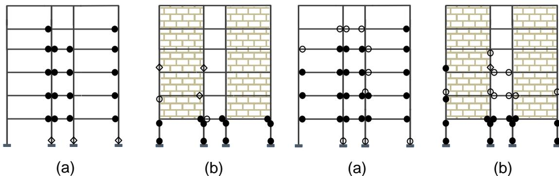
Fig. 6. The plasticity development of FRAME1 (a) without the infills, (b) with the infills.
