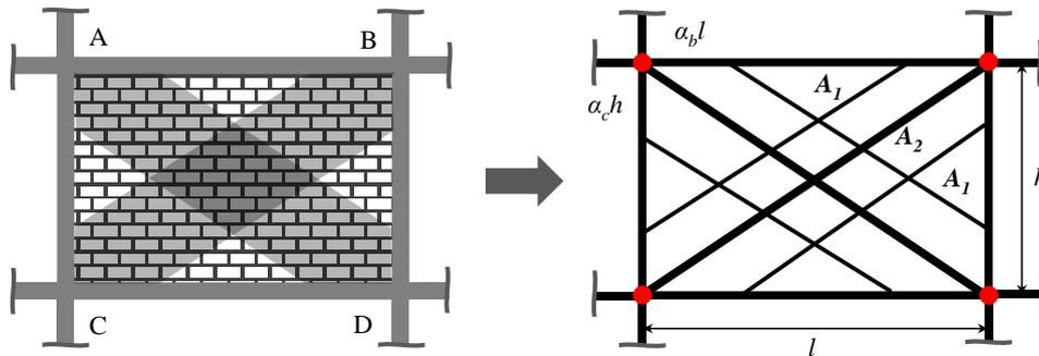
Fig. 1. The three-strut model for infilled frame.
