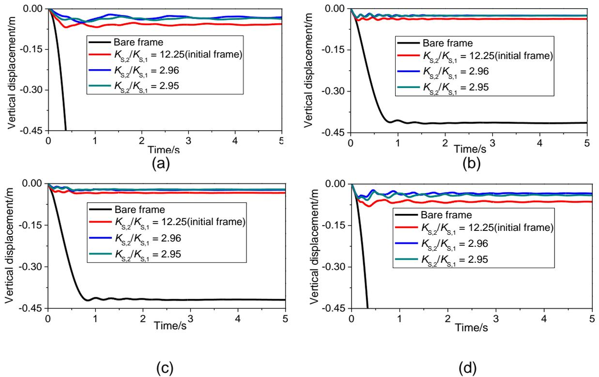
Fig. 19. Displacement time-history of FRAME1 with the earthquake-induced damage (a) Column A removed, (b) Column B removed, (c) Column C removed, (d) Column D removed.
