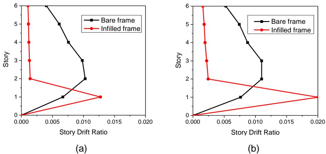
Fig. 5. Comparison of story drift ratios (a) For FRAME1, (b) For FRAME 2.
