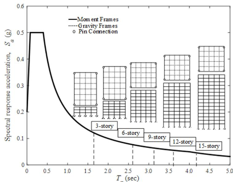
Figure 1. Design spectral response acceleration of IMFs assigned to SDC  $C_{max}$
