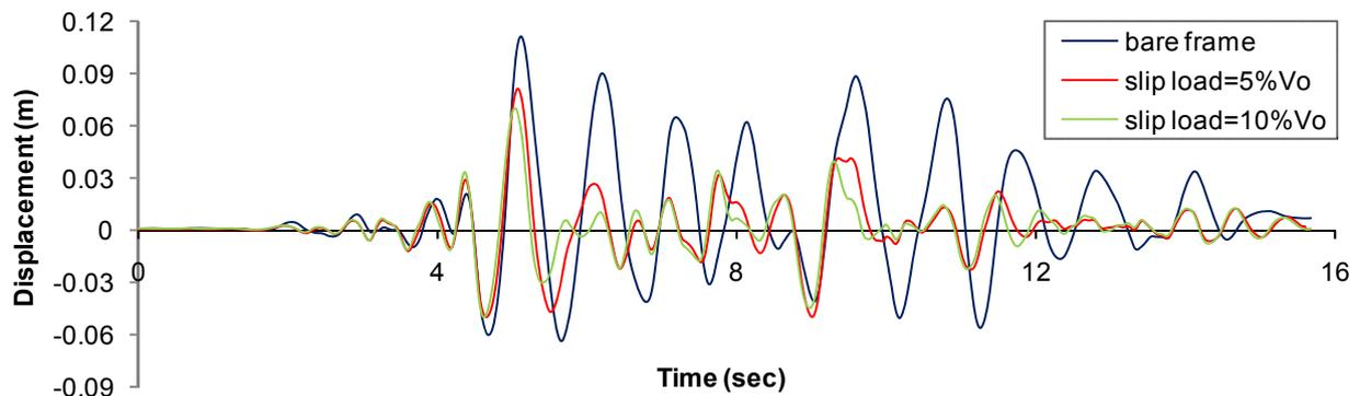
Fig. 13 Top displacement of the second frame
