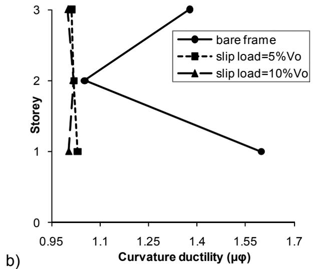
Fig. 8 Average curvature ductility of the a) first frame and b) second frame
