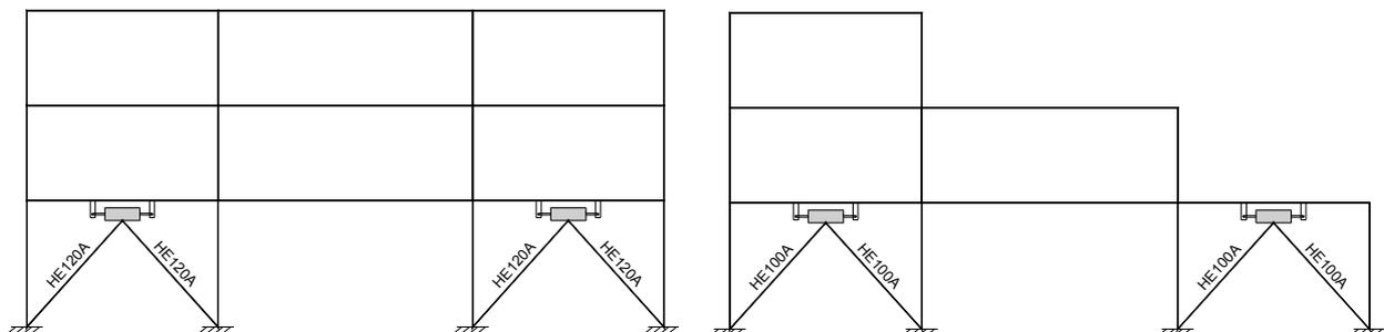
Fig. 4 Retrofitted frames
