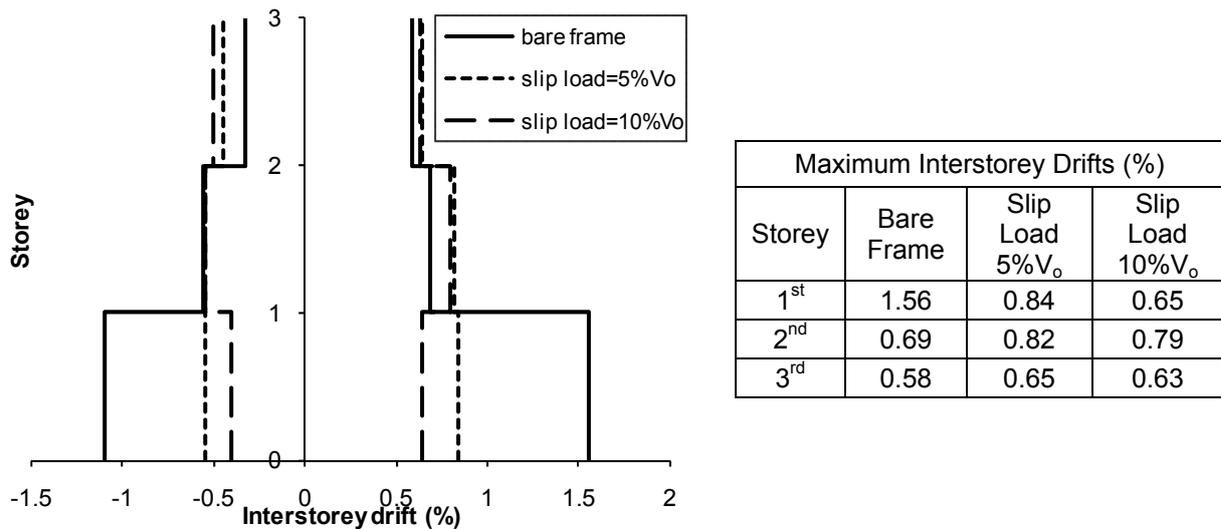
Fig. 11 Interstorey drifts of the first frame
