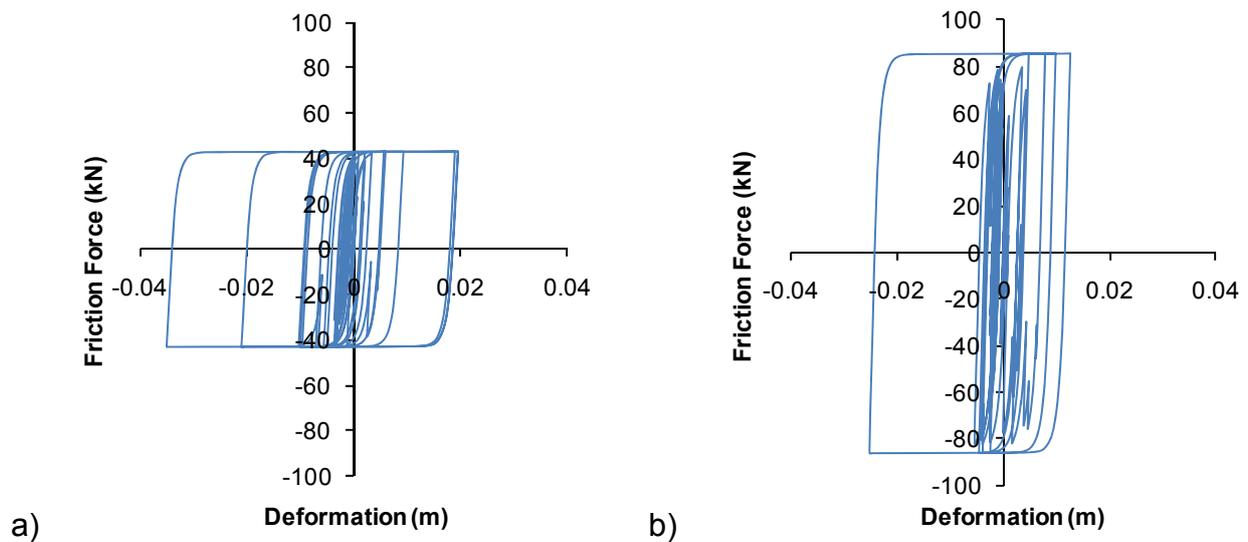
Fig. 12 Hysteresis behavior of friction damper for slip load a)  $5\%V_o$  and b)  $10\%V_o$
