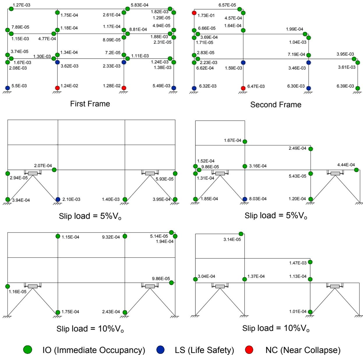
Fig. 5 Average values of plastic hinge rotations  $\theta_{pl}$  for both structures
