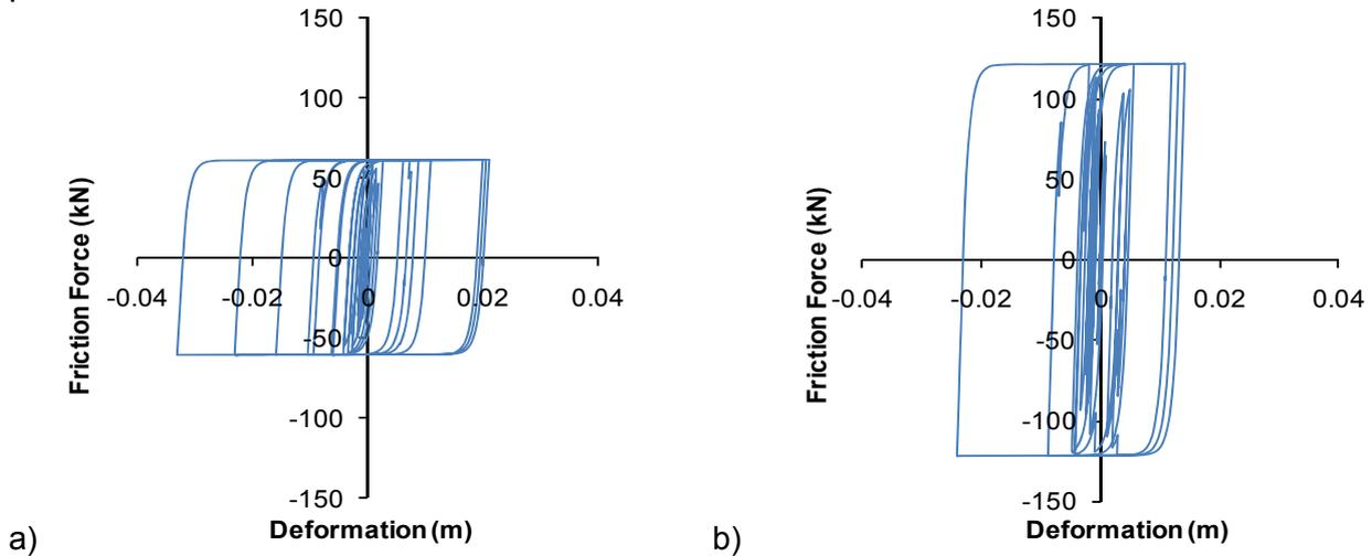
Fig. 9 Hysteresis behavior of friction damper for slip load a) 5% $V_o$  and b) 10% $V_o$ .
