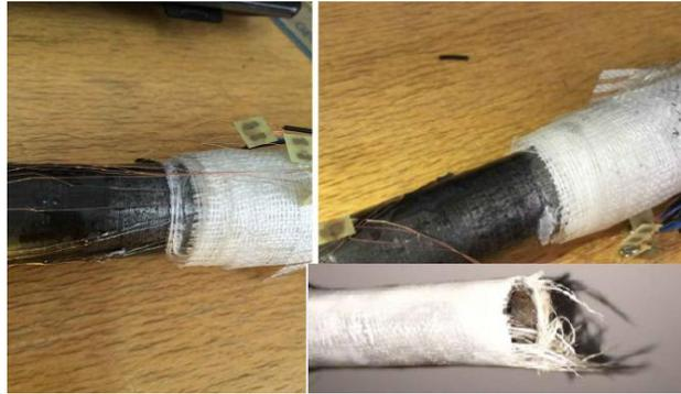
Fig.6 Failure surfaces and failure modes
