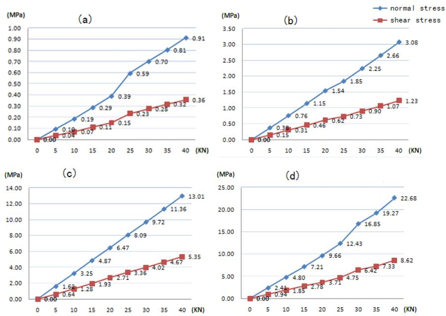
Fig.4 Load–normal/shear stress
