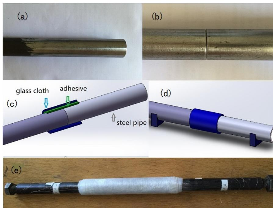
Fig.1 Aspects of the adhesive bonding processes: (a) surface preparation, (b) protecting ends, (c) adhesive application and (d) clamping and curing (e) The bonded specimen.
