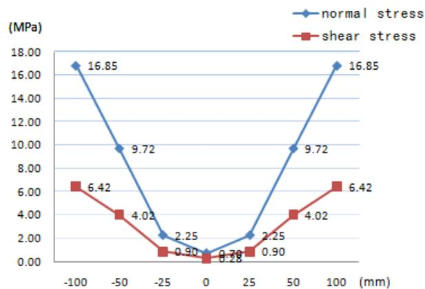
Fig.5 Location–normal/shear stress
