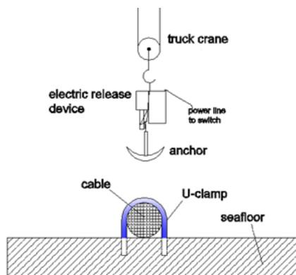
Fig. 2 Schematic diagram of test system
