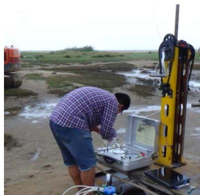
Fig. 1 Soil properties test with DMT
