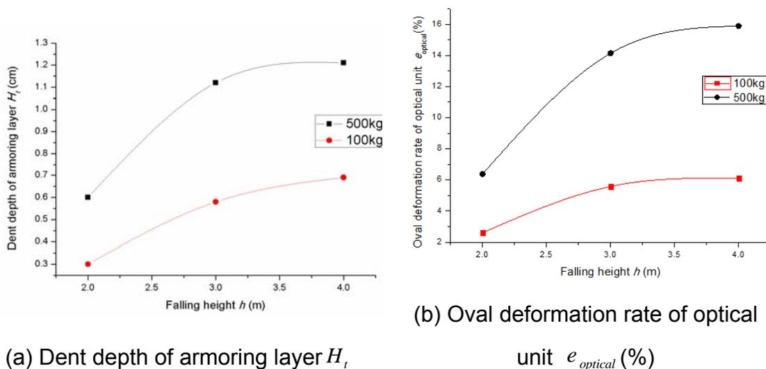
Fig. 5 Relationship of cable deformation with anchor weight and falling height
