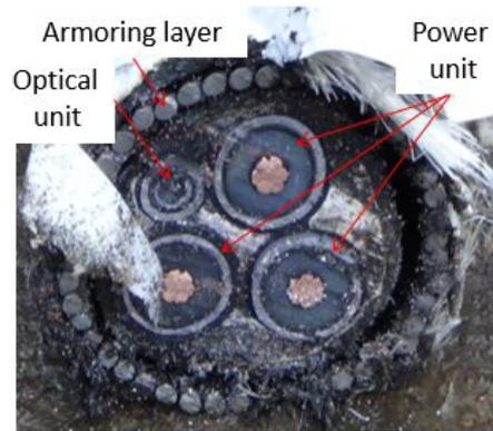
Fig. 4 (a) Cross section of cable specimen
