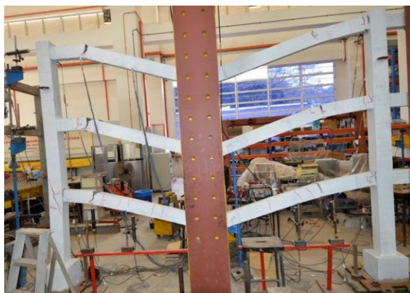
Fig. 4 Failure mode of Specimen NS
