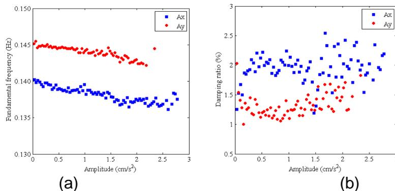
Fig 9. Amplitude dependencies of building modal parameters: (a) natural frequencies; (b) damping ratios
