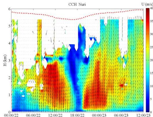
Fig 3. Variations of 30-min mean wind profiles in form of filled color contour (the dotted line stands for variations in air pressure)
