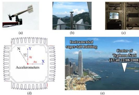
Fig 2. Some sensors of the SHM system installed in a super-tall building: (a) propeller anemometer; (b) GPS antenna; (c) control system; (d) locations of the accelerometers and orthogonal directions X and Y; (e) locations of the instrumented super-tall building and the center of Typhoon Nuri around 17:40 on 22 August, 2008.
