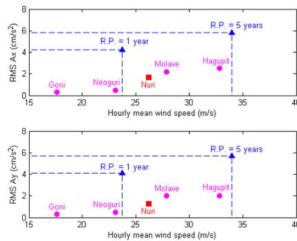
Fig 11. Variation of maximum RMS acceleration responses with hourly mean wind speeds measured at Waglan Island
