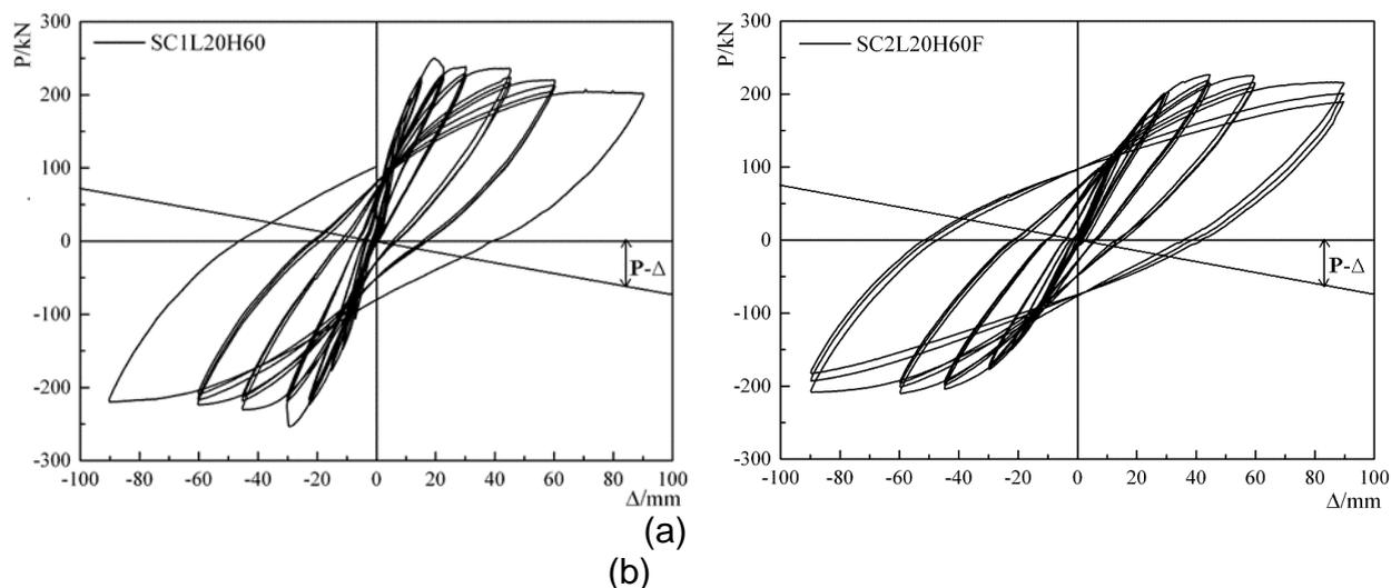
Fig. 2. Cyclic response of columns: (a) Specimen 1; (b) Specimen 2
