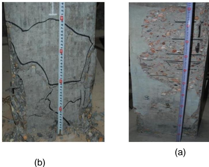
Fig 1. Damage state following earthquake and fire: (a) flexural cracking after seismic loading; (b) spalling damage after fire loading
