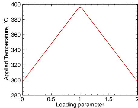
Fig. 2 Temperature loading cycle.
