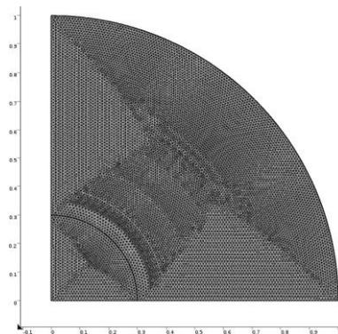
Fig. 1 Finite element mesh for the composite disc with the inclusion radius  $a = 0.3$  m. Axis labels are in units of m.
