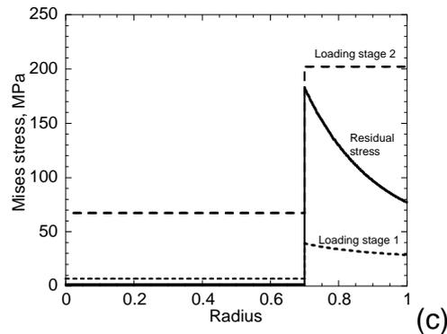
Fig. 3 Residual effective stress after a temperature loading cycle for the disc's inclusion radius being (a)  $a=0.1$ , (b)  $a=0.3$  and (c)  $a=0.7$  m.
