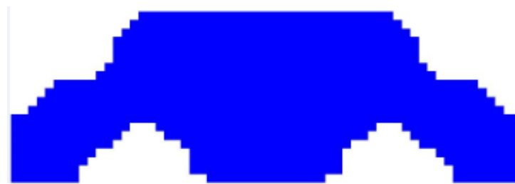
Fig. 4. The optimal topology of the plane stress plate obtained by the proposed method
