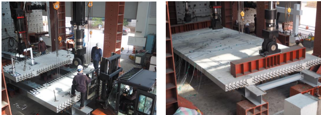
Fig. 4 Test of a two-girder composite bridge using precast decks
