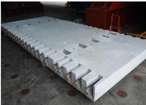
Fig. 2 Precast deck module with ribbed loop joints
