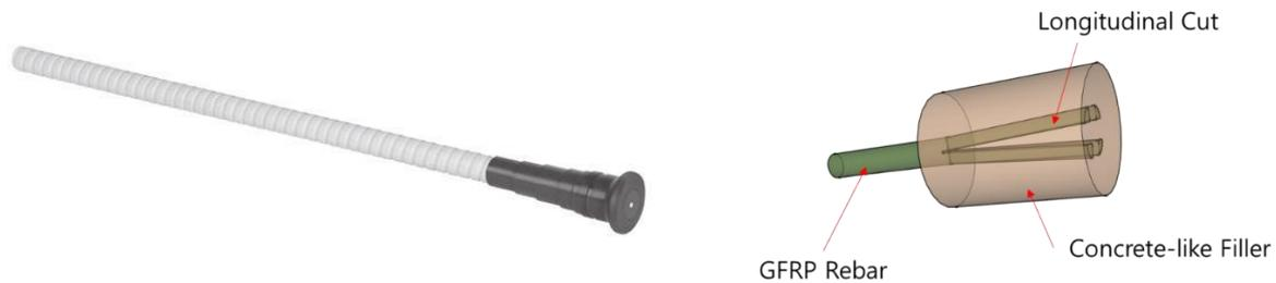
**Fig. 1** Plastic headed GFRP rebar of ComBAR([www.schoeck-combar.com](http://www.schoeck-combar.com)) and concrete-headed GFRP rebar proposed in this study
