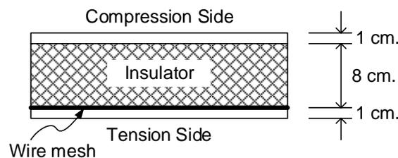
**Fig. 1** Details of test specimens
