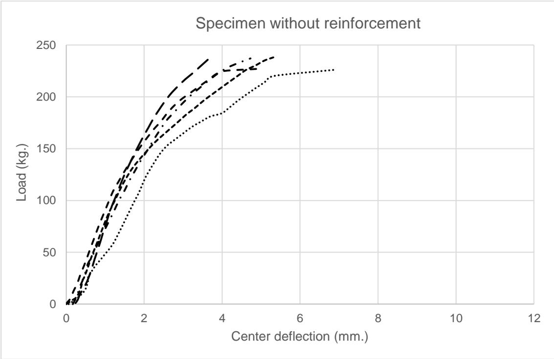
**Fig. 4** Flexural behaviour of specimens without reinforcement
