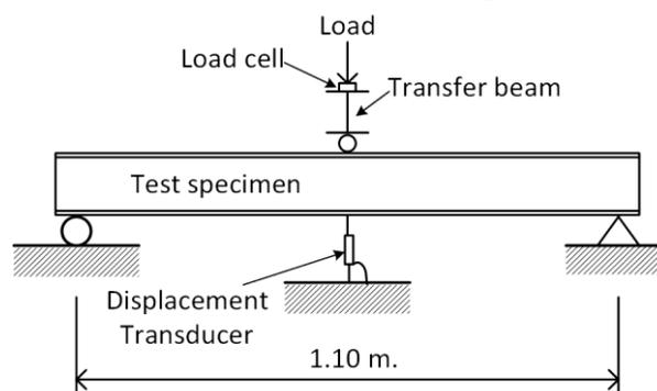
**Fig. 2** Details of centre point load flexural test
