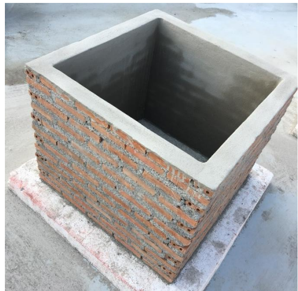
Fig. 2 Details of masonry wall test specimen
