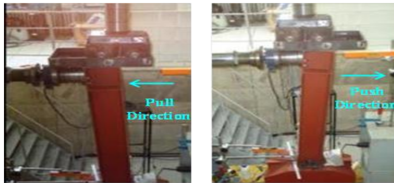
Figure 9. Application of a cyclic lateral displacement at the pile top (a) pull, (b) push direction
