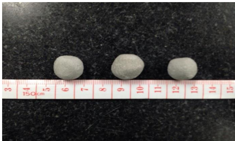
Fig. 1 The pellets of cold-bonded lightweight aggregate
