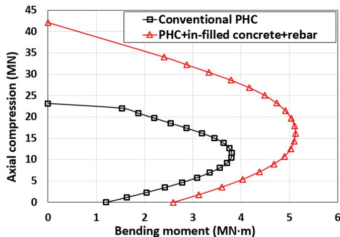
Fig.2 P-M interaction of pile specimens
