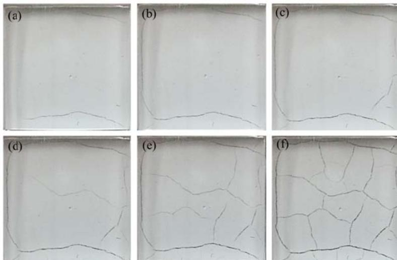
Fig. 2 Crack propagation process on the top surface of 10mm thickness specimen
