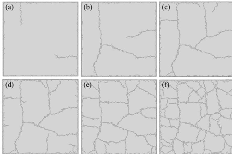
Fig. 5 Crack propagation process on the top surface of 10mm thickness model
