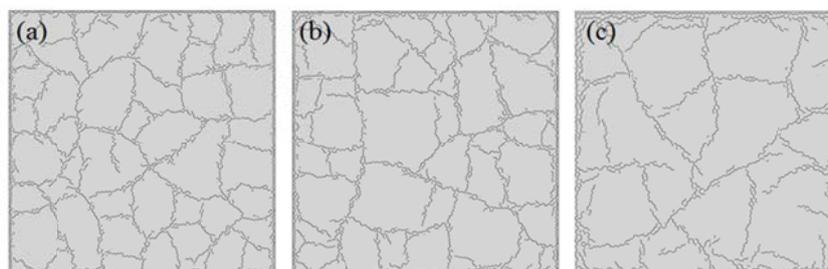
Fig. 4 The final crack patterns formed on the top surface of the analysis models with different thickness. (a) 5mm, (b) 10mm, (c) 20mm
