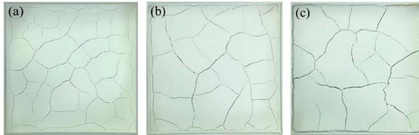
Fig. 1 The final crack patterns formed on the top surface of the specimens with different thickness. (a) 5mm, (b) 10mm, (c) 20mm
