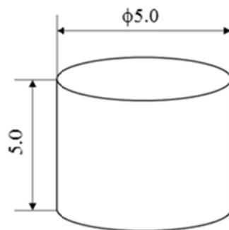
Fig. 1: Dimensions of specimen for thermal desorption analysis, in mm.
