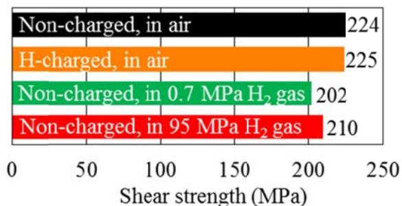
Fig. 4: Nominal shear stress at final fracture.
