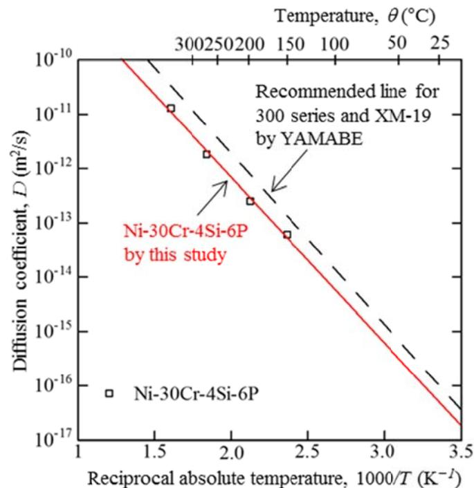
Fig. 3: Arrhenius plot of the diffusion coefficient.
