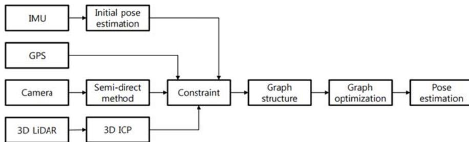
**Fig. 1** Graph-based SLAM algorithm (developed by Prof. H. Myung (KAIST))
